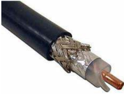
Construction of Belden 9913 semi-air-spaced cable. A spiral of polyethylene filament separates the solid inner conductor from the polyethylene tube. This tube is wrapped in polyester/aluminum foil, with tinned copper braid as the outer conductor.
