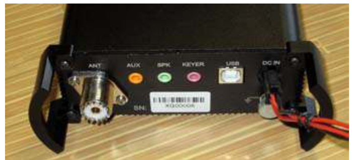
Back of the X-108 transceiver with connectors (L to R) for antenna, aux., speaker, key, USB, DC power and ground.
