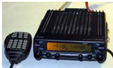
Icom IC-2710H VHF/UHF transceiver had only one of its three display lamps working.
