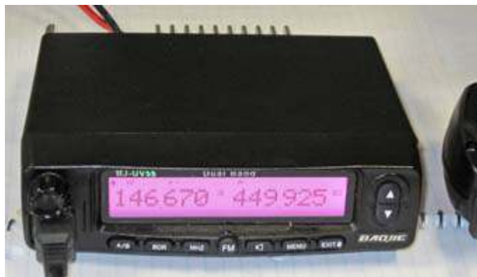
Baojie BJ-UV55 dual-band mobile transceiver, programmed by W2CH for the PCARA repeaters.
