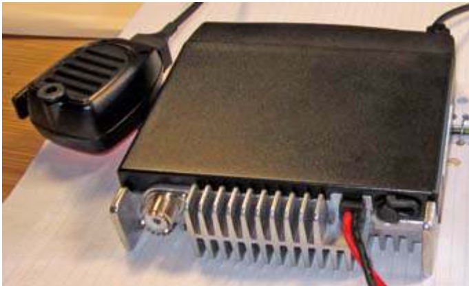
Rear view of Baojie BJ-UV55 showing (L to R) the antenna connector, heat-sink, power cord and external speaker connector.
