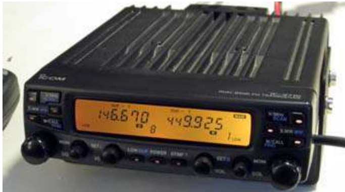
Icom IC-2710H, now fully illuminated. Front panel has separate controls for VHF left side and UHF on right side.
