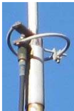
Cable connection and base ring of the old AR-2 Ringo.
