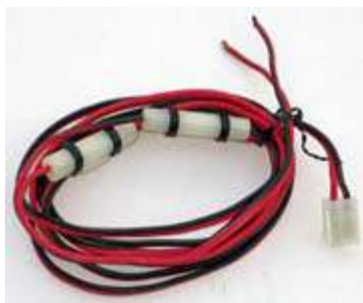
Smelly cable from the Icom IC-2710H.
