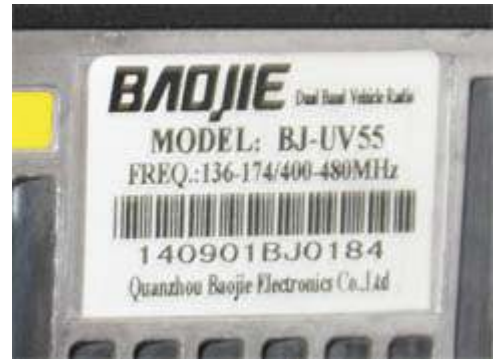
Label on the bottom of the transceiver indicates the frequency coverage.
