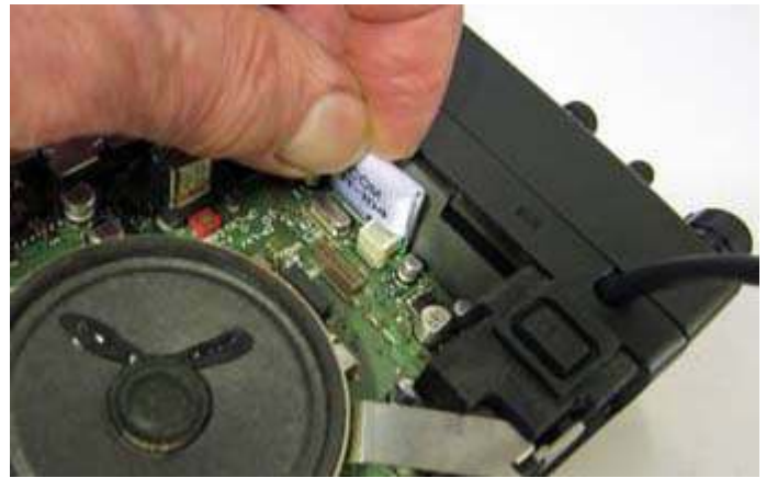
Insertion of UT-104 Tone Squelch Unit into the miniature socket on the main circuit board of the IC-2710H.
