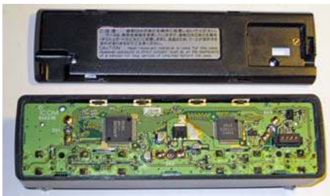
Control unit for the IC-2710H with back cover removed.
