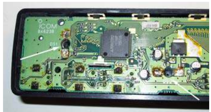
Control unit after burnt-out lamps DS1 and DS2 had been removed (arrowed), ready for the new lamps.
