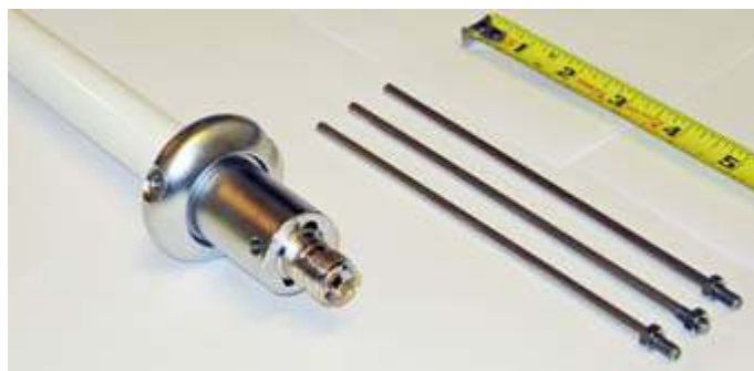
Base of the Comet GP-1 antenna showing the SO-239 socket and the three radials, ready to be screwed in.
