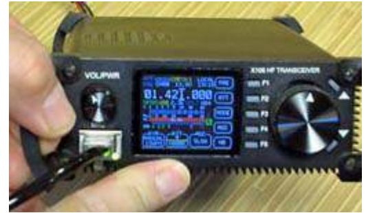
The Xiegu X-108 HF transceiver is a tiny radio, measuring only 4 3/4" x 1 3/4" x 7".
