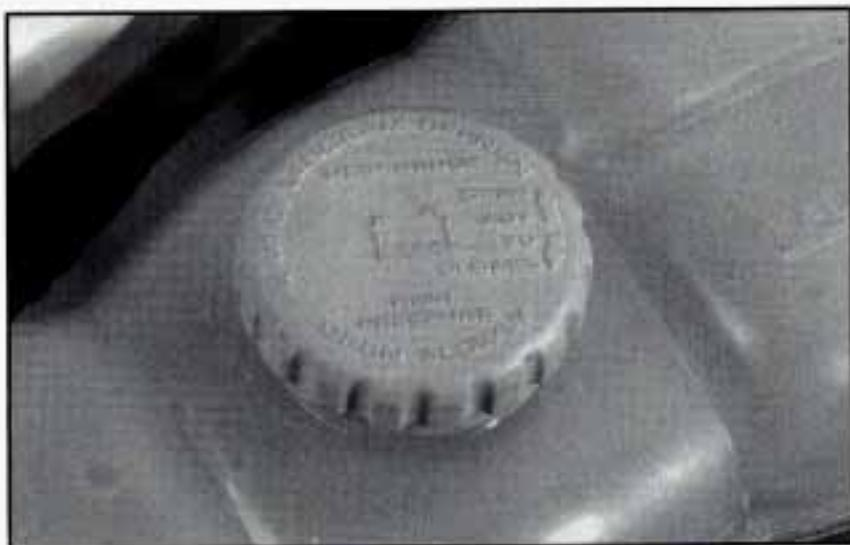
5. Then replace the pressure cap. Be sure the pressure cap is tight.
