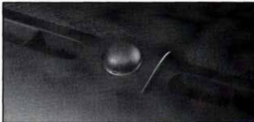
The light sensor for the twilight sentinel is located in the center of the front defogger grille. If you cover the sensor, it will read “dark” and the parking lamps and low-beam headlamps will come on.
