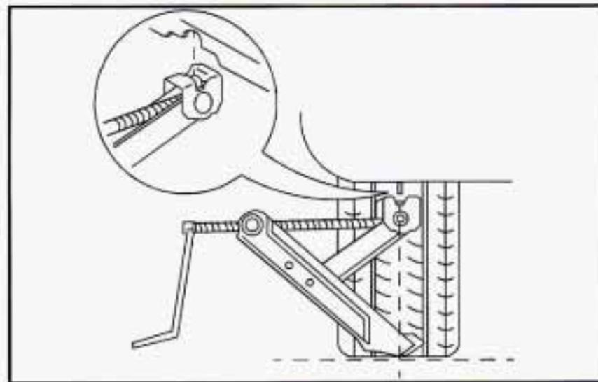
The base of the jack must line up vertically with the hoisting notch (jack contact point) on the vehicle's frame, nearest the flat tire. Then, raise the jack lift head until it is firmly set into the hoisting notch.
