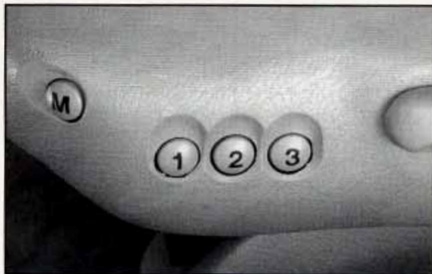
Adjust the driver's seat to a comfortable position. Also adjust the interior and exterior mirrors. Press memory button "M" and memory button "1" at the same time.
