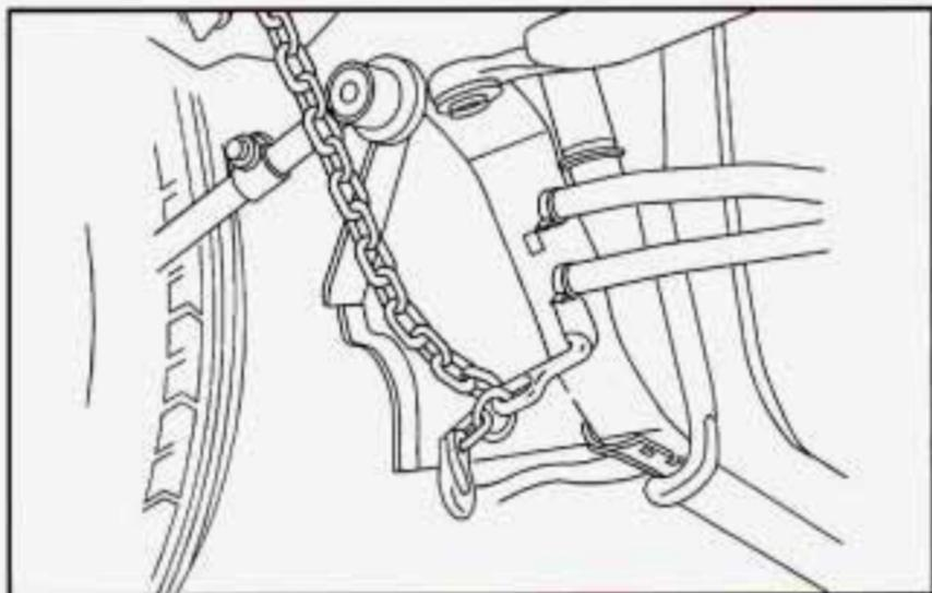
Attach R-hook chains on both sides, in the slotted holes in the bottom of the frame rails, behind the front wheels. These slots are to be used when loading and securing to car-carrier equipment.
