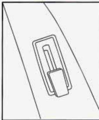
The latch is located on the side of the passenger's front seatback closest to the door, above the manual recliner and lumbar support control. Lift the latch and push the passenger's seatback toward the front of the vehicle to provide extra storage in your vehicle, if needed.
