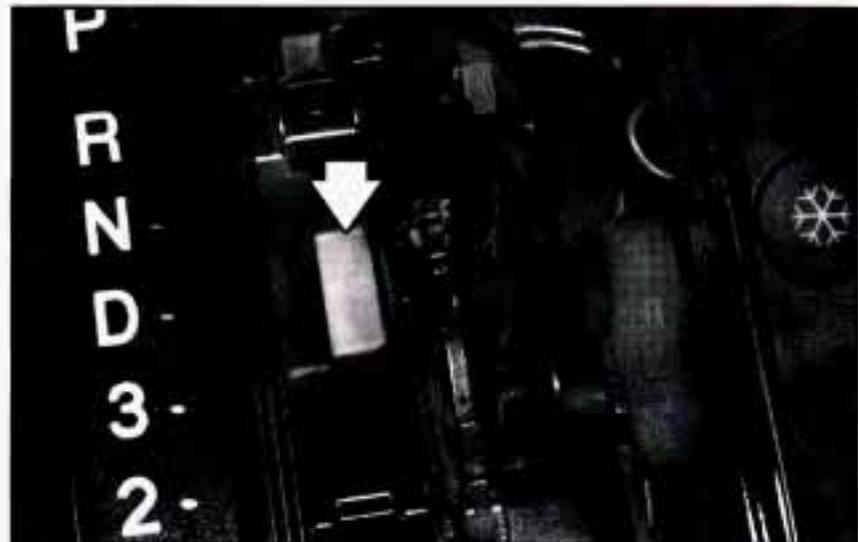
6. At the bottom of the shift lever, you will see a yellow tab. With one hand, push the tab to unlock the shift lever.
