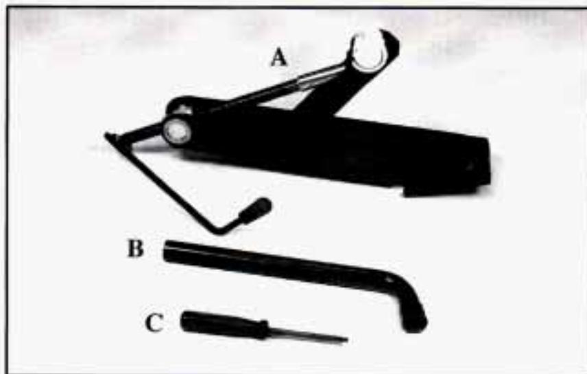
The tools you'll be using include the jack (A), the wheel wrench (B) and the screwdriver (C).
