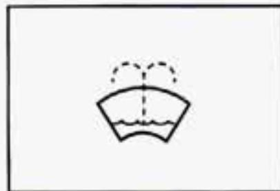
This light will come on when you turn on the ignition and the windshield washer fluid container is less than one-third full.
