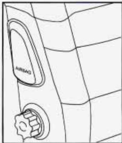
If your vehicle has side impact air bags, it will say AIR BAG on the air bag covering on the side of the driver's and right front passenger's seatback closest to the door.
