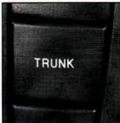
To use this feature, your vehicle must be in PARK (P). Press the trunk release button located on the center console next to the radio to open the trunk.
