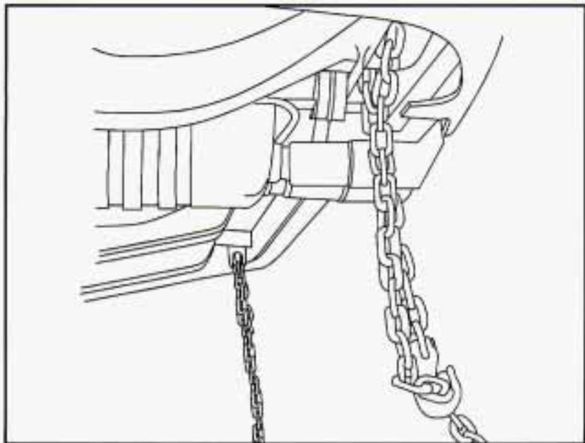
Attach a separate safety chain around the bumper energy absorbing shock/unit on the left side of the vehicle and another safety chain on the right side tow hook.
