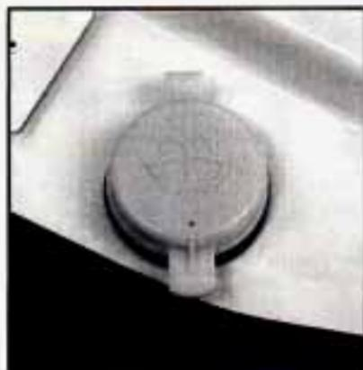
The windshield washer fluid reservoir is located behind the front grille on the driver's side of the engine.
