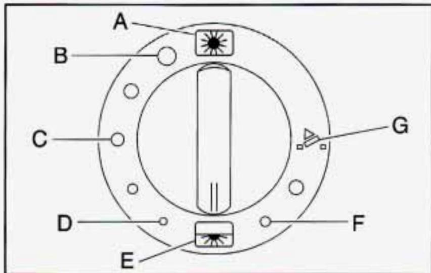
Turning the control dial to position A fully opens the glass panel and sunshade. The sunshade can also be opened by hand. If you want to stop the roof in a partially opened position, turn the control dial to any position between A and E. The positions range from about 25 percent open to approximately 80 percent open. Turn the dial to position E to fully close the glass panel. To close the sunshade, manually pull it forward.
