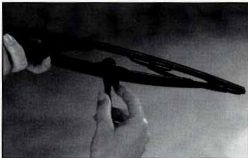
2. Press the tabs together and pull the wiper blade assembly down enough to release it from the "J" hooked end of the wiper arm. Slide the assembly away from the arm.
