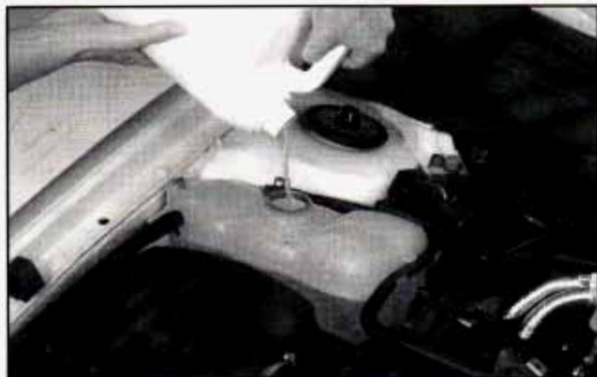
3. Then fill the coolant surge tank with the proper mixture, up to the KALT/COLD line (seam).
