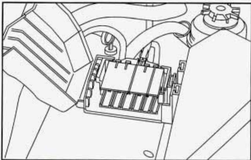
This fuse block is attached to the engine compartment relay center located on top of the battery. Simply lift the lid to open. If you have any questions about the power distribution fuse block, consult your dealer.
