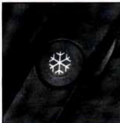
Press this button to provide more traction when you are starting on ice or other slippery surfaces. It only operates when the shift lever is in DRIVE (D). The button is located next to the shift lever on the console.
