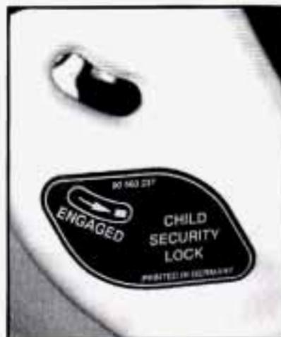
Your vehicle is equipped with rear door security locks that help prevent passengers from opening the rear door of your vehicle from the inside. The lock is located on the rear edge of each rear door. To use this lock:
