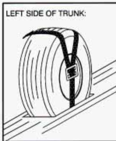
Put the flat tire in the trunk where the spare is stored (driver's side wheel well). Secure the flat tire with the straps that are used to hold the spare in place.
