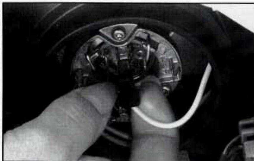
3. Remove the plug connector from the bulb.
