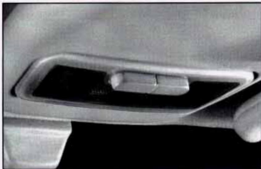
These lamps are located in the front overhead console (near the windshield). Press either button to turn the driver's or passenger's side lamp on and press the button again to turn the lamp off.
