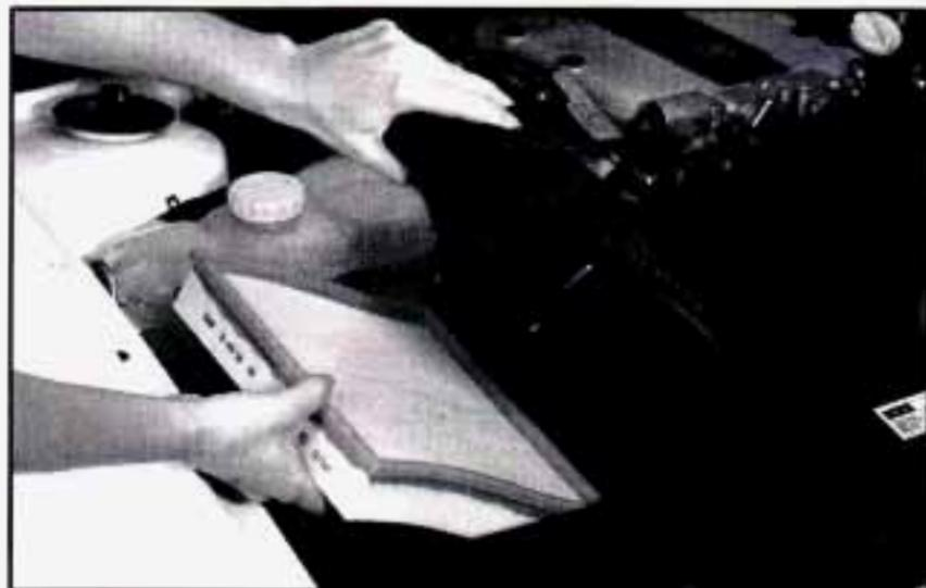
4. Lift the lid, take out the air filter and remove any loose debris that may be found lying in the air cleaner base.
