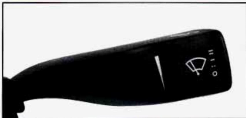
**WIPER:** Move the lever on the passenger's side of the steering wheel up and down to control the wipers.
