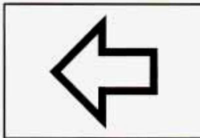
This arrow on the instrument panel will flash in the direction of the turn or lane change.
