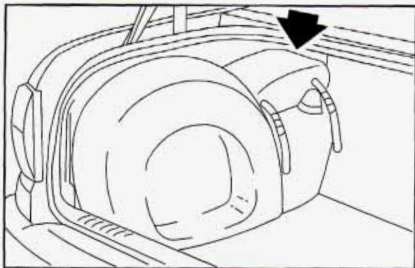
The head restraint should be stored securely on the driver's side of the trunk as shown.
