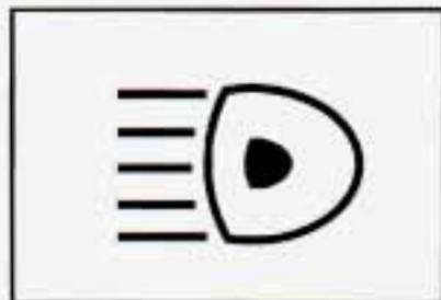
This light on the instrument panel will be on, indicating high-beam usage.
