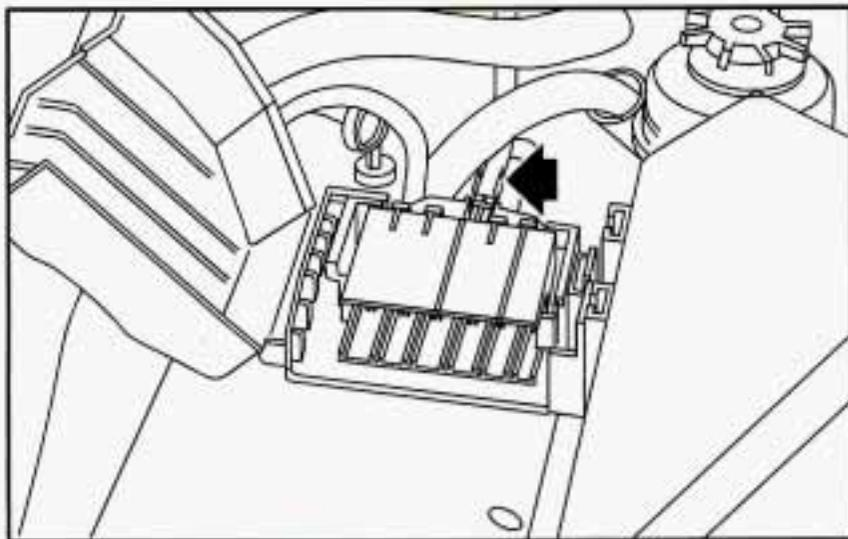
4. Open the hoods and locate the batteries. You'll also need to open the power distribution fuse block cover to access the positive (+) terminal on the battery (see arrow).
