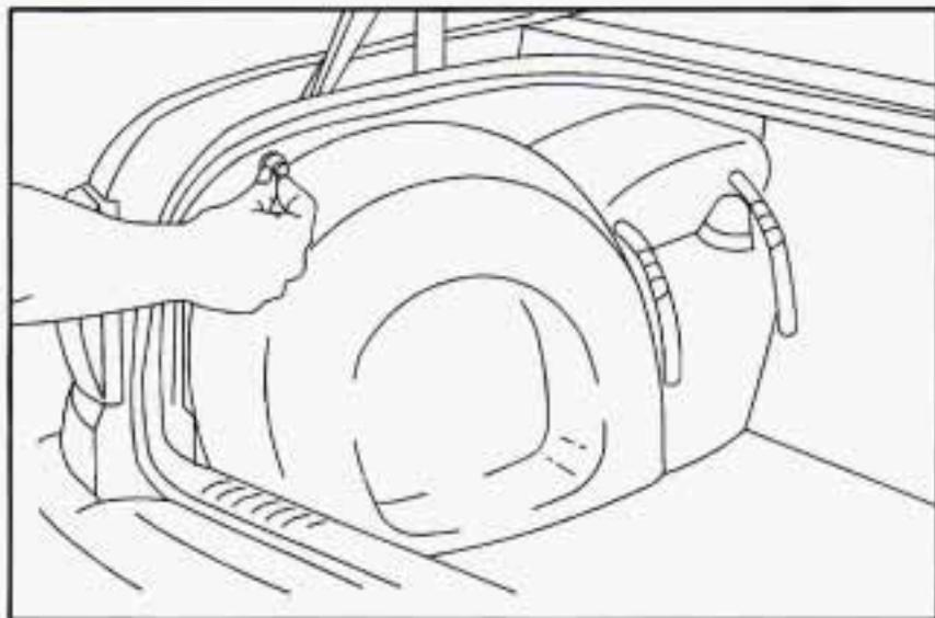
The equipment you'll need is in the trunk. On the driver's side of the trunk is the spare tire. Pull the fasteners on the spare tire cover to access the tire.
