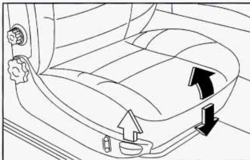
To tilt the front portion of the seat cushion up or down, lift the seat lever located on the side of the seat cushion closest to the door. Release the lever to lock the seat into place.
