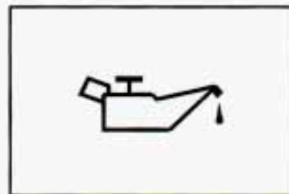
The oil light goes on when you turn the key to ON or START. It goes off once you start the engine. That's a check to be sure the light works.
