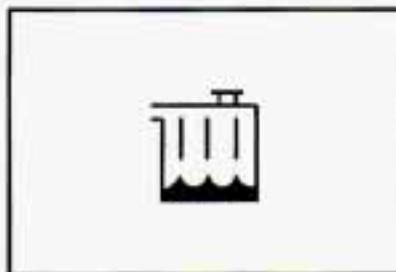
If the light comes on, it means you're low on engine coolant.
