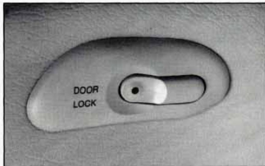
Press the power door lock switch to lock or unlock all of the doors at once.
