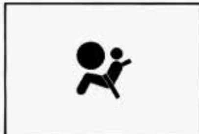
This light will come on when you start your engine, and it will flash for a few seconds. Then the light should go out. This means the system is ready.
