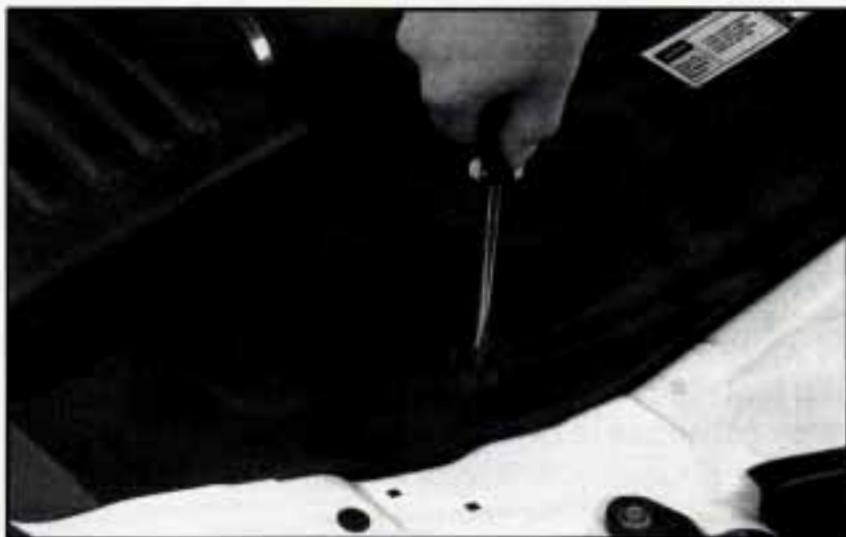
1. With a screwdriver, unscrew the fastener on the headlamp cover and then remove the cover to gain access to the headlamps. Note that the inner bulb is for the low-beam headlamp and the outer bulb is for the high-beam headlamp.
