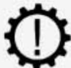
This light comes on briefly when the ignition is turned on. If the light remains on or lights up while driving, there may be a fault in the automatic transmission. Have your vehicle serviced.
