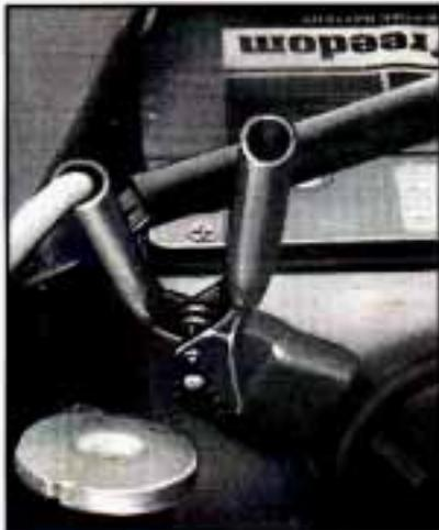
7. Don't let the other end of the positive cable touch metal. Connect it to the positive (+) terminal of the good battery.
