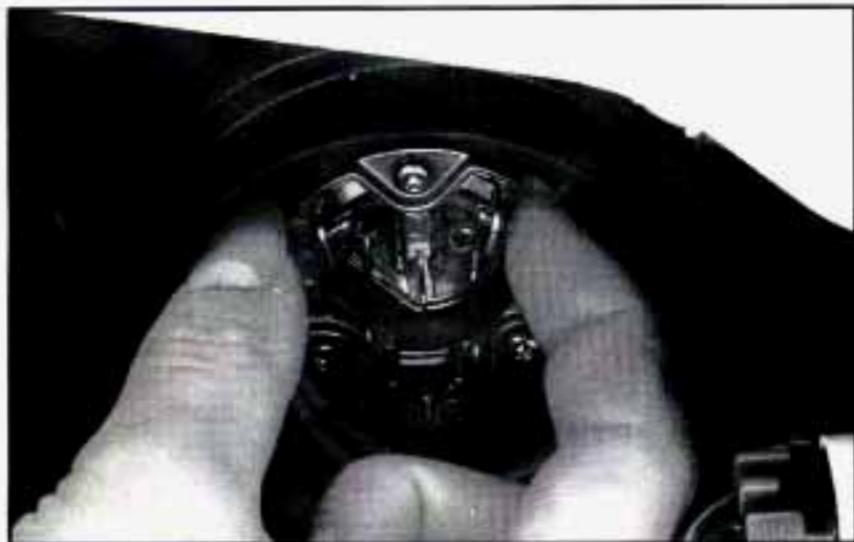
4. Squeeze the retaining clip together and then pull away from the bulb assembly.
