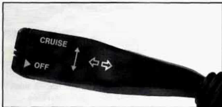
With cruise control, you can maintain a speed of about 25 mph (40 km/h) or more without keeping your foot on the accelerator. This can help on long trips. Cruise control does not work at speeds below about 25 mph (40 km/h).
