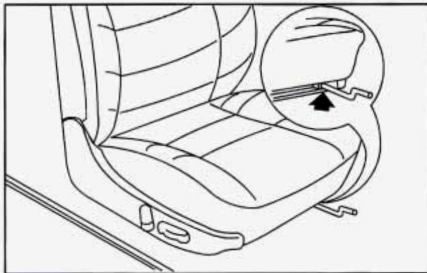
If a failure in the power supply system occurs, the power seats can be manually adjusted by inserting the crank handle into the slot located below the seat cushion (as shown in the above illustration). Turn the crank handle to the right until you've reached your desired seating position (note that manually moving the seat requires turning the crank handle many times).
