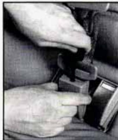
Insert a key or a similar object into the slot as shown to unlatch the buckle. Move the belt to the side so it is not in your way.
