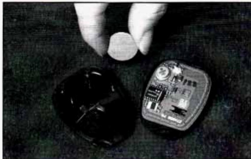
2. Remove the battery and replace it with a CR2032 battery. Using the wrong size battery can damage the transmitter. Make sure the battery is positioned with the "plus" (+) facing down.
