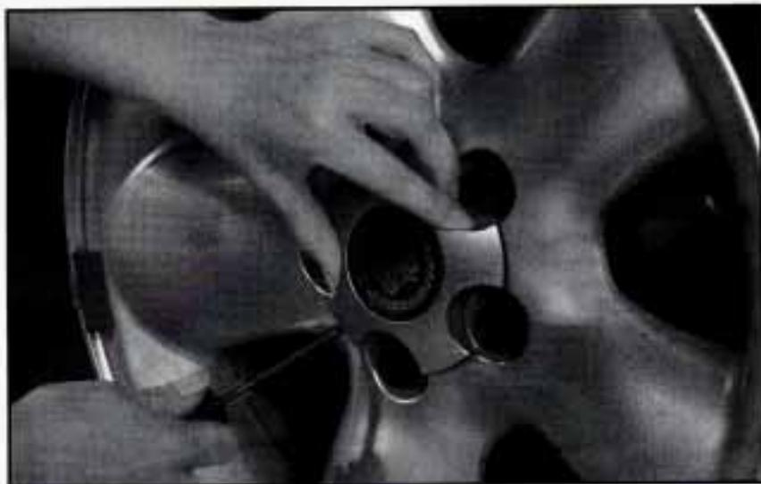
Using the flat end of the screwdriver, gently pry the wheel cover off. Be careful not to scratch the wheel edge.
