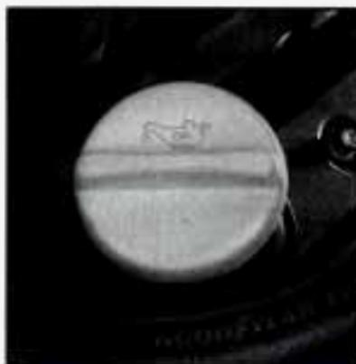
The oil fill cap is located behind the engine oil dipstick and next to the engine block on the driver's side of the engine. Turn the cap to the left to remove it.
