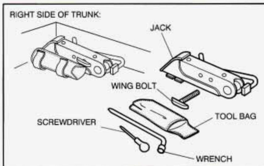
The jacking tools are stored on the passenger's side of the trunk behind the panel with the red pull handle. Make sure these tools are properly secured when not in use.
