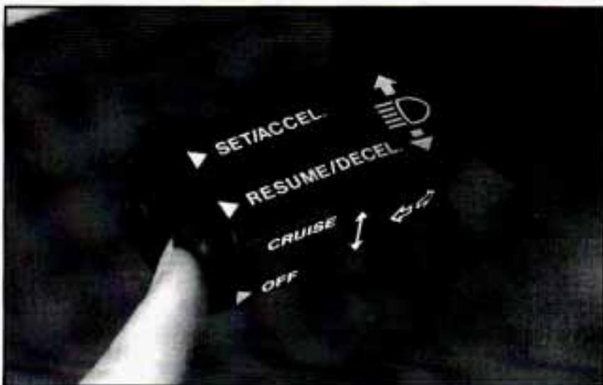
Setting the cruise control at a desired speed and then applying the brake will end the cruise function. Once you're going about 25 mph (40 km/h) or more, you can press the RESUME/DECEL button briefly to reset. This returns you to your desired preset speed.
