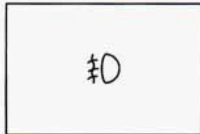
This light on the instrument panel will come on when the fog lamp button is pressed.
