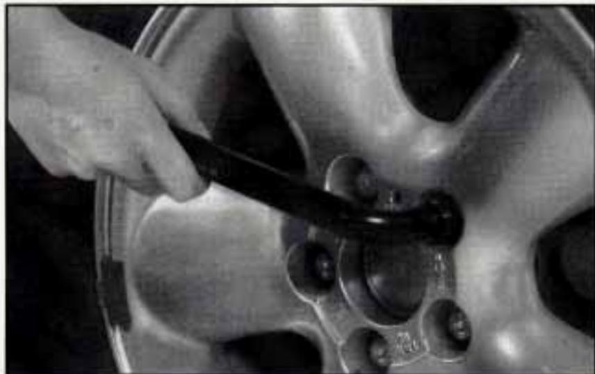
2. Using the wheel wrench, loosen all of the wheel bolts. Don't remove them yet.
