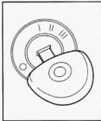
With the key in the ignition switch, you can turn the switch to four different positions.
