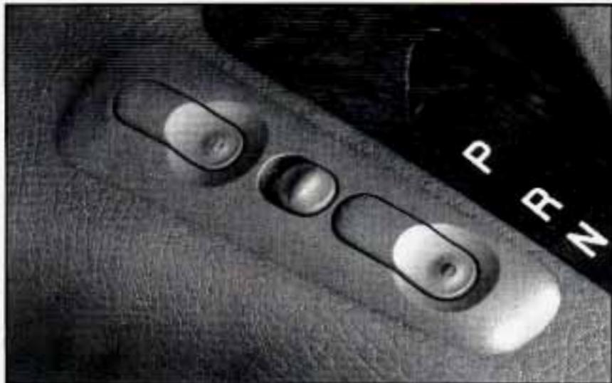
The controls are located next to the console shift lever. Tap the controls forward or rearward to raise or lower the windows in increments. To express-open the window, press the control rearward for about one second and then release. If you want to stop the window as it is lowering, tap the control. Pressing the control forward for about one second and then releasing it will express-close the window.
