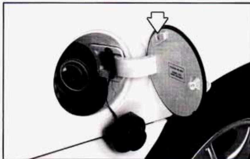
Your vehicle may or may not have a tethered fuel cap. Hang the fuel cap inside the fuel door as shown by the arrow.
