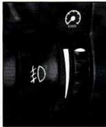
Use the fog lamps for better vision in foggy or misty conditions. Press this button to turn the fog lamps on and press the button again to turn the lamps off. (The fog lamps only work when the parking lamps or the low-beam headlamps are on.)
