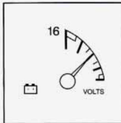
You can read battery voltage on the voltmeter. If it reads less than 12 volts or more than 16 volts while the engine is running, and it stays there, you may have a problem with the electrical charging system.
