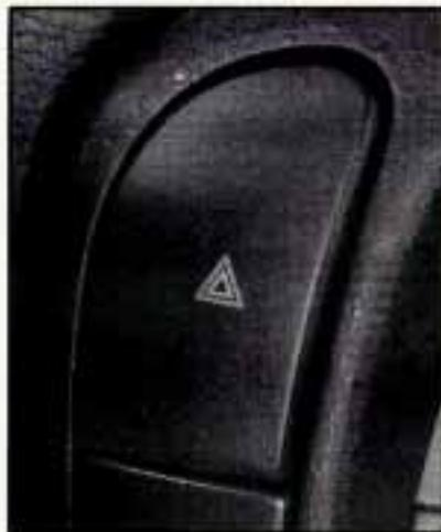
Pressing this button on the center console makes the front and rear turn signal lamps flash on and off. The indicator light on the button also flashes. Pressing the button again turns the flashers off. The flashers work regardless of the key position.
