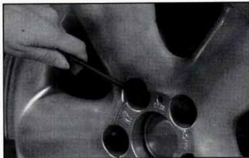
1. If you have the five-spoke wheel, use the flat end of the screwdriver to pry off the five black plastic wheel bolt caps. Be careful not to scratch the wheel edge. (This step does not apply to the seven-spoke wheel.)
