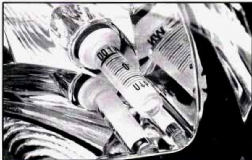
2. Check the vertical aim for each headlamp and adjust it as necessary. The vertical aim adjustment screw is located on the outboard side of the headlamp assembly. You can see the level through the headlamp assembly. Turn the vertical aiming screw until the bubble in the level is centered at 0 (zero).
