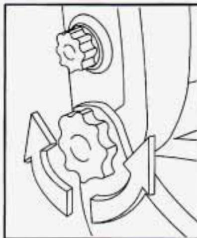
This feature is found on the passenger's seat only. The manual recliner control is located on the side of the passenger's seatback closest to the door, below the lumbar control. See "Manual Lumbar Support" earlier in this section.
