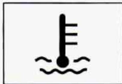
This light tells you that the engine has overheated. If this light comes on, you should stop the vehicle and turn the engine off as soon as possible. A warning chime should also sound if this light comes on.
