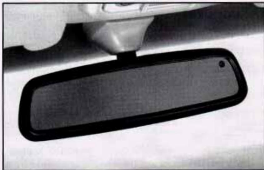
This mirror automatically changes to reduce glare from headlamps behind you. A photocell on the back of the mirror senses when it is becoming dark outside. Another photocell built into the mirror surface senses when headlamps are behind you.
