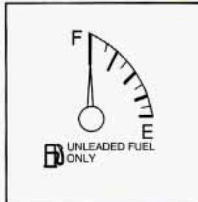
The fuel gage shows approximately how much fuel is in the tank. It works only when the ignition is in ON.
