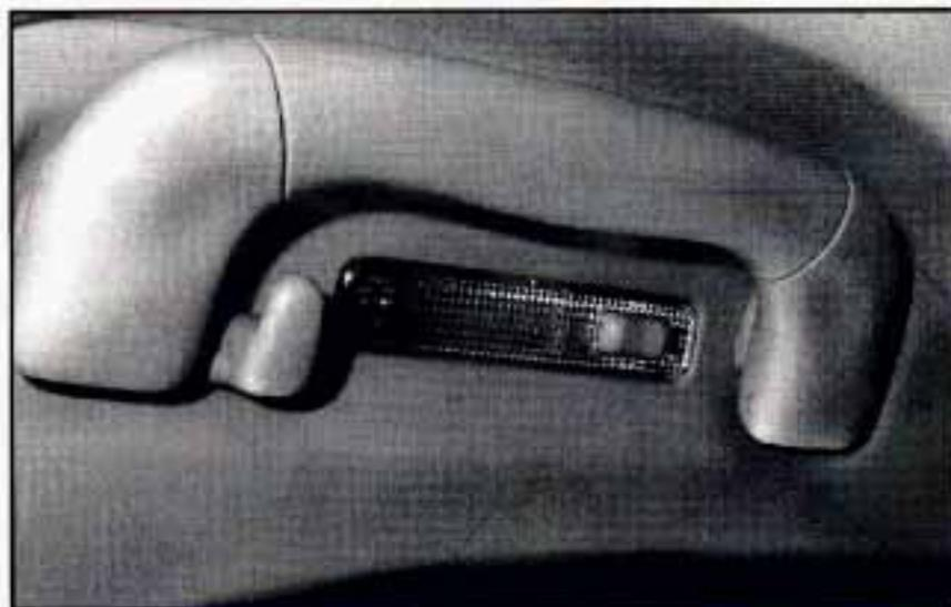
The rear reading lamps are located above each rear door. These lamps and the interior courtesy lamps come on when any door is opened and it is dark outside.
