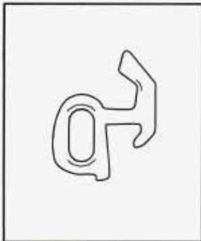
This is a sample of an R-hook. It is the only type of hook that may be used to tow your vehicle from the front or from the rear.
