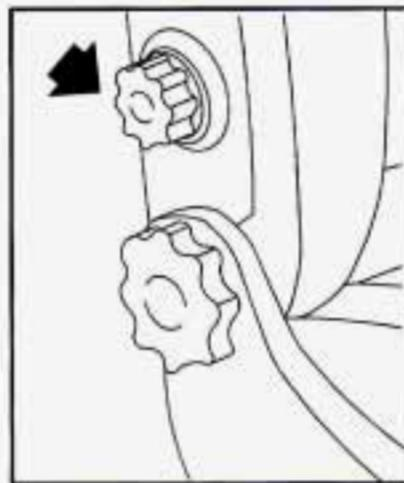
The lumbar control is located on the side of each front seatback closest to the door. The control provides additional support to your lower back and works independently of other seat controls.
