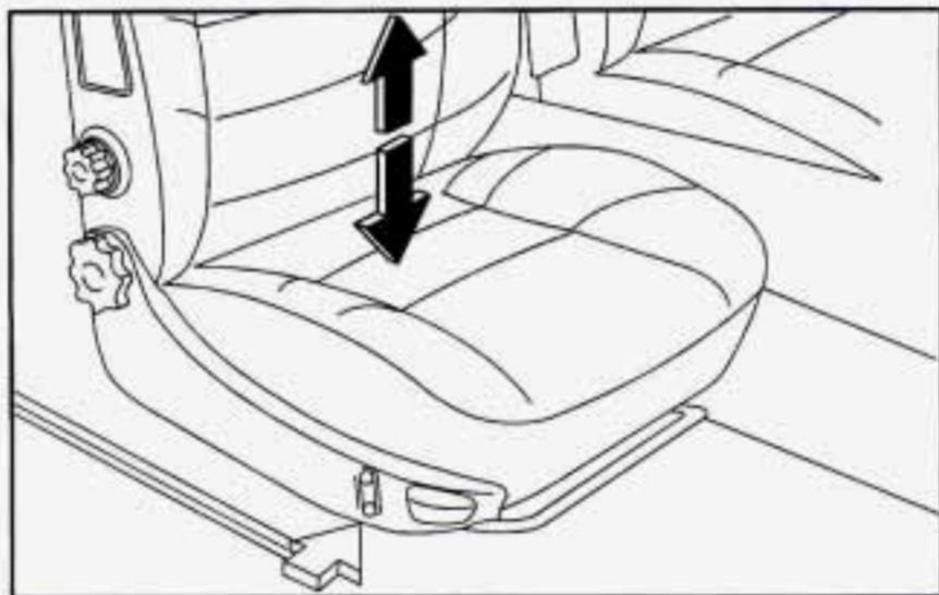
To raise the seat cushion up or down, press one of the rocker switch buttons located on the side of the passenger's seat cushion closest to the door. The top button raises the seat cushion and the bottom button lowers the seat cushion.
