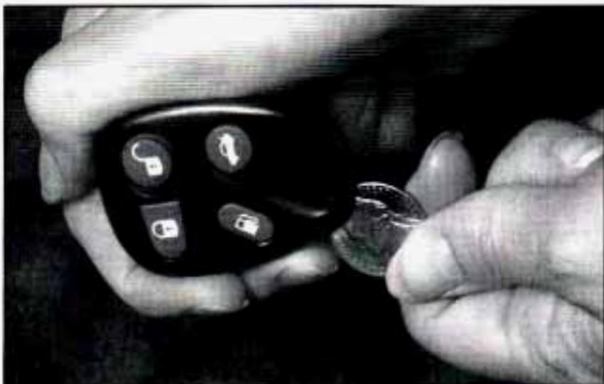
1. Use a coin to pry open the transmitter.
