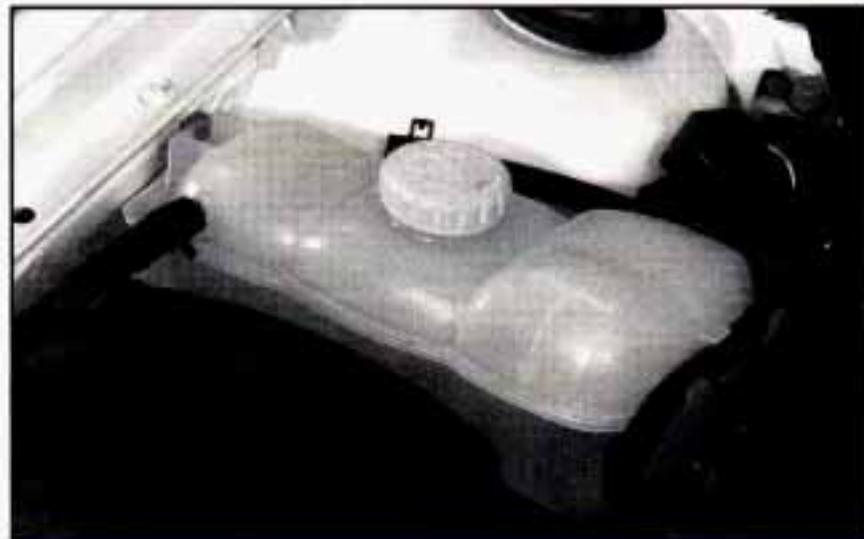
The coolant level should be at or slightly above the KALT/COLD line (seam).
