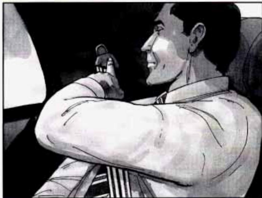
Press the release button and move the height adjuster to the desired position. After you move the adjuster to where you want it, try to move it down without pressing the release button to make sure it has locked into position.
