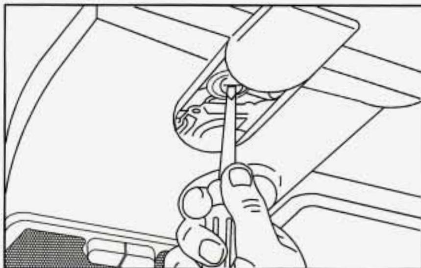
If a failure in the power supply system occurs, the sunroof can be manually closed by inserting a screwdriver into the slot as shown. Turning the screwdriver to the left will close the sunroof.
