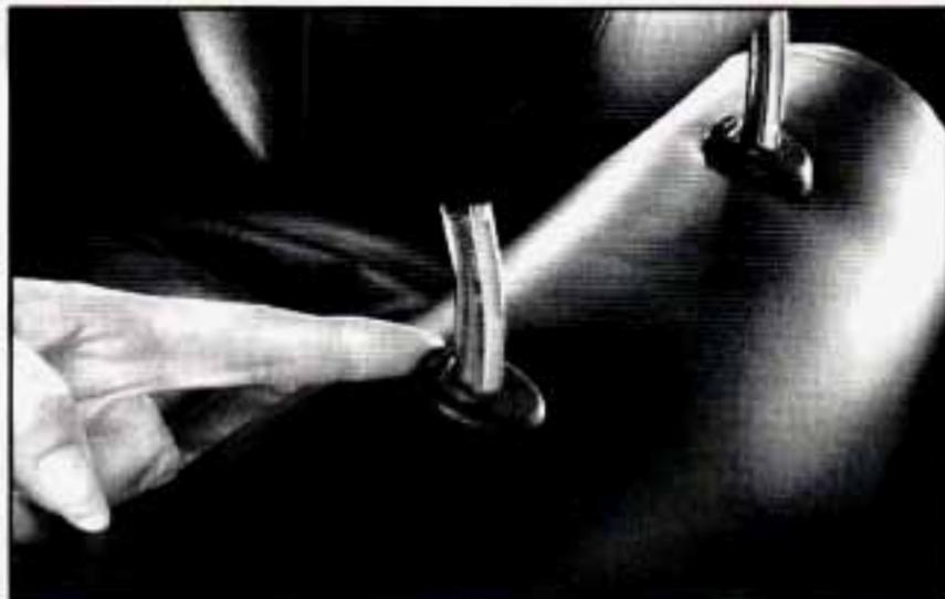
For more cargo space or to fold down the front passenger's seat, you may need to remove the head restraint. Press both release buttons at the top of the seatback and slide the head restraint out of the height adjust tubes.
