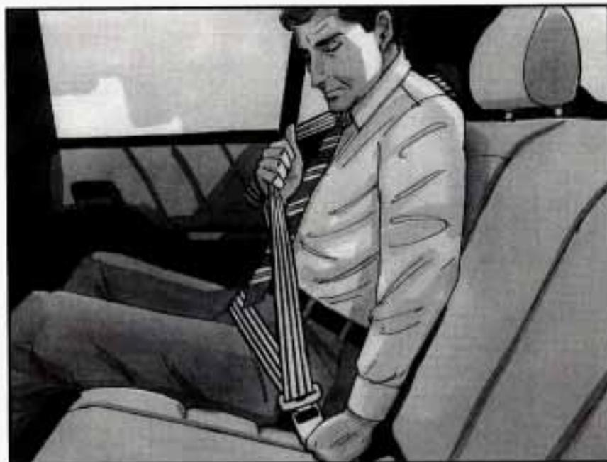
3. To make the lap part tight, pull down on the buckle end of the belt as you pull up on the shoulder part.
