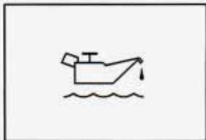
If the low oil level light on the instrument panel comes on, it means you need to check your engine oil level right away. For more information, see "Low Oil Level Light" in the Index.
