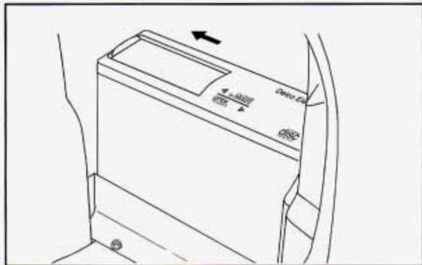
Close the door by sliding it all the way to the left. When the door is closed, the changer will begin checking for discs in the magazine. This will continue for up to one and a half minutes, depending on the number of discs loaded.
