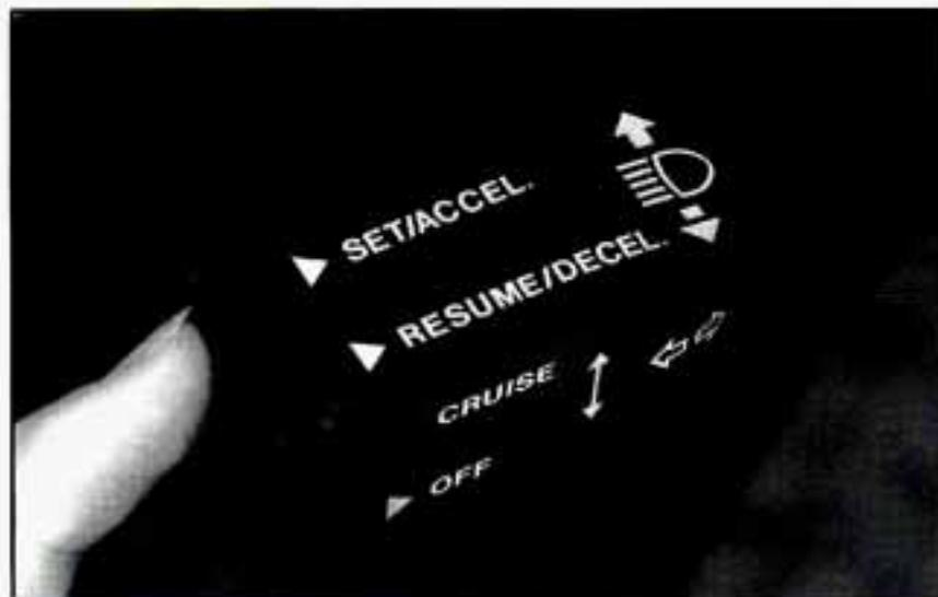
2. Press the SET/ACCEL button at the end of the lever and release it.
