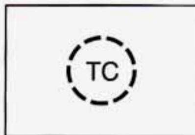
The warning light will flash when the system senses a traction change.
