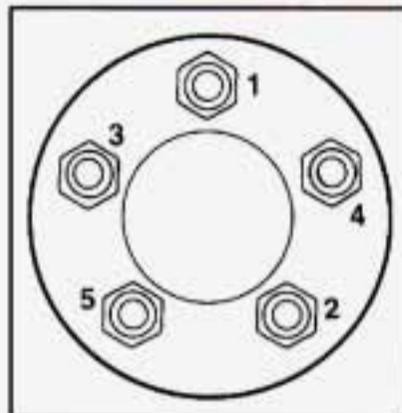
12. Tighten the wheel bolts firmly in a criss-cross sequence as shown.
