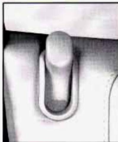
From inside your vehicle, slide the lock lever down to lock the door. To unlock the door, slide the lock lever up.
