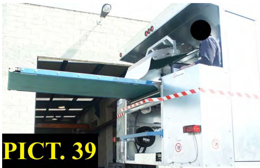
The caging belt is in its full extension ( pict. 39 ).
