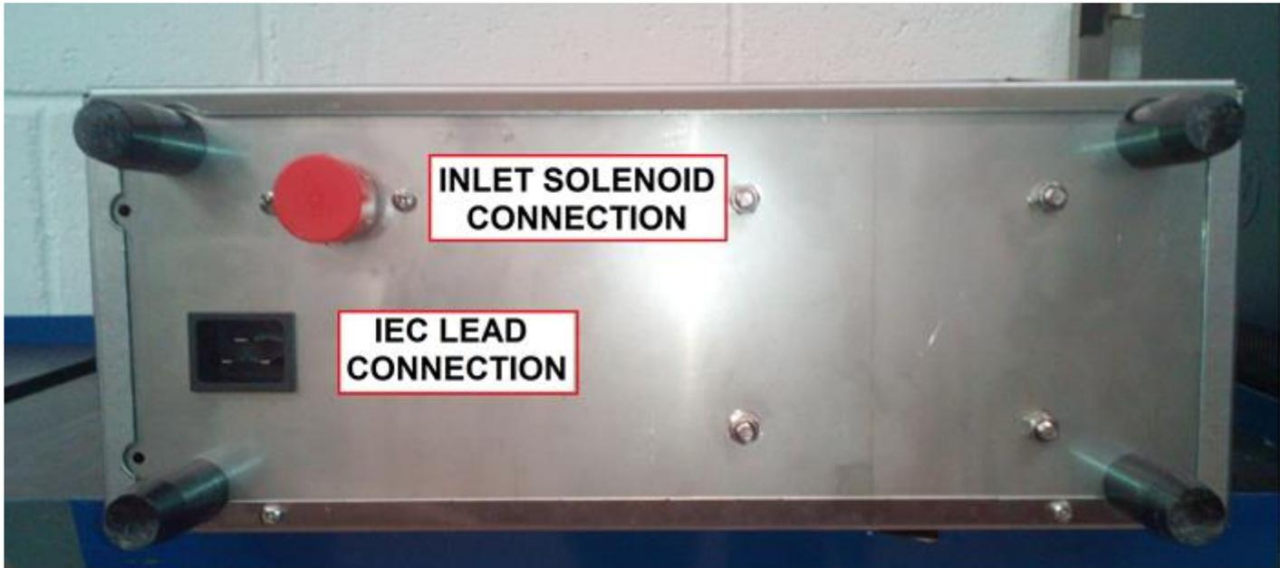
Figure 8 - Base of SP9 Undercounter Unit
