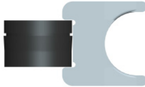
Figure 4-10: Replace Mesh in Filter Holder
