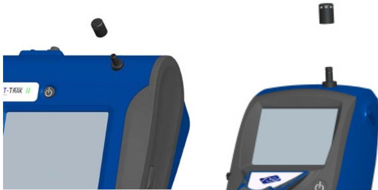
Figure 2-3: Putting on Inlet Cap
