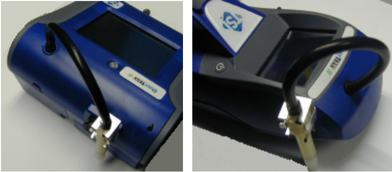
Figure 2-5: Installing Door-Oliver Cyclone
