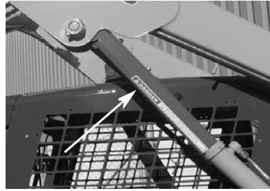
Figure 4 Lift Arm Support Device Engaged
