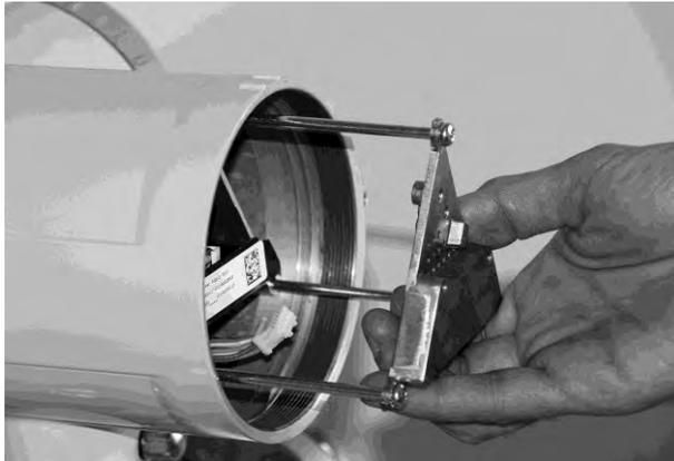
8. Using tool no. 1, pull out the triangular housing with the power supply cassette.
