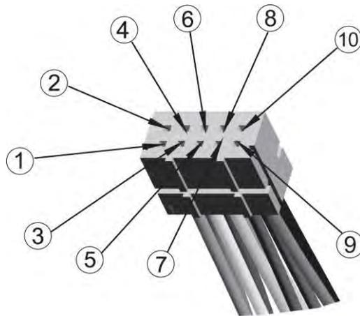
Figure 3-6 Sensor cable connector pins
