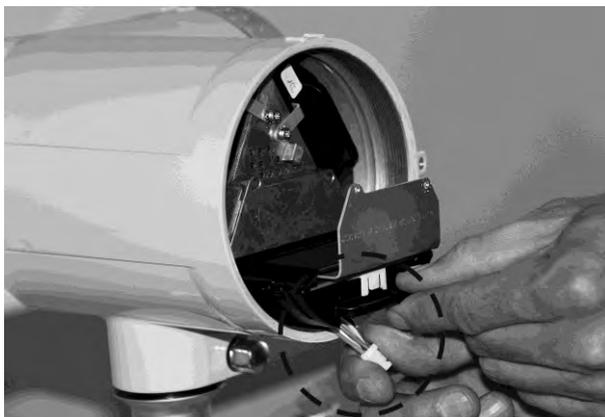
2. Reconnect cassette cable plug until the catch clicks. Push the cassette in place, and tighten the two screws.
