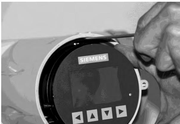
4. Using tool no. 8, remove the screw holding the I/O cassette.
