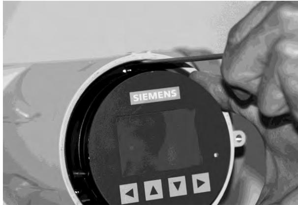
4. Using tool no. 8, remove the two screws that hold the sensor interface cassette.
