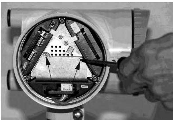
2. Pull out the sensor interface module to the position shown in the photo.
