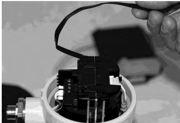
3. Disconnect the cable plug as shown in the photo.
