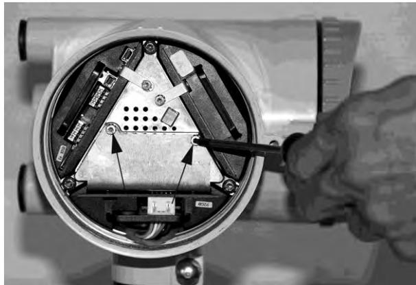
5. Pull out the sensor interface module to the position shown in the photo, and disconnect the cable plug while lifting the catch.
