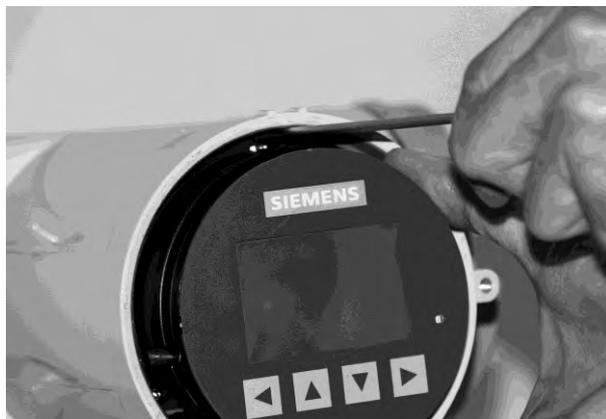
3. Remove the SensorFlash by pressing and releasing it.
