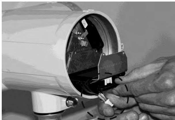
2. Reconnect cassette cable plug until the catch clicks. Push the cassette back in place, and tighten the two screws.
