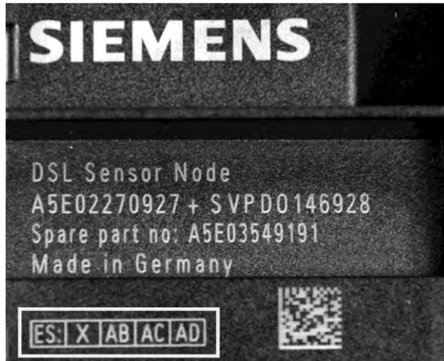
Figure 5-6 The revision no. is stated on the product label. The "X" marks the revision state. In this example the revision state is "ES AA".
