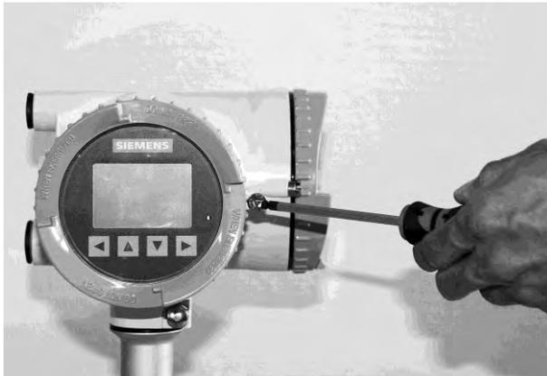
3. Carefully remove display and cable plug.
