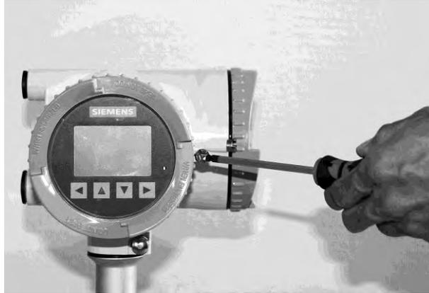
2. Carefully remove display and cable plug.
