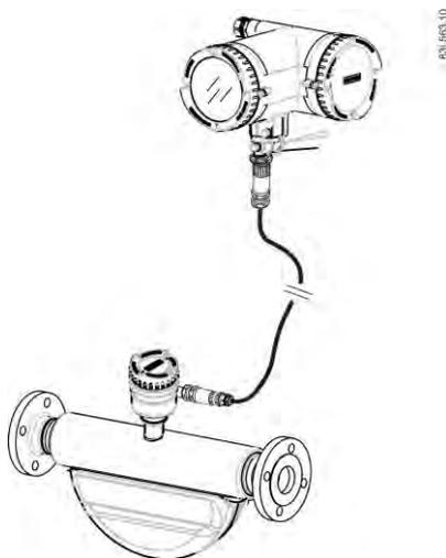
Figure 2-2 Remote version with M12 connection
