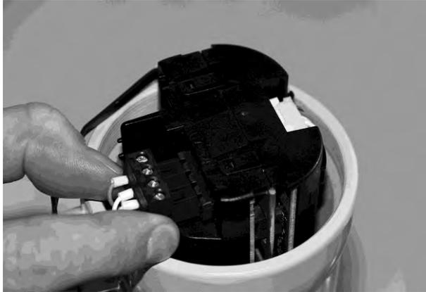
4. Using tool no. 8 remove the screw that holds the DSL cassette.
