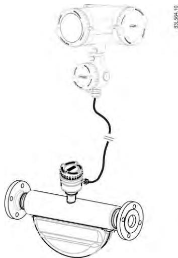
Figure 2-3 Remote version with terminated cable
