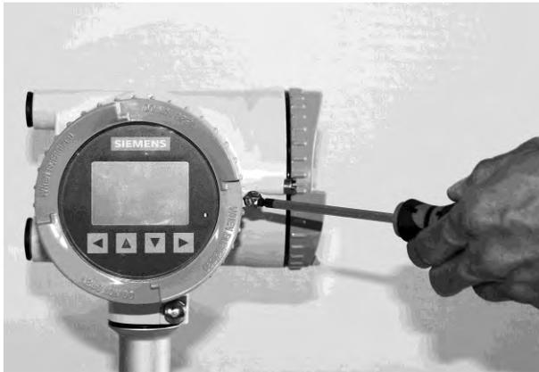
3. Carefully remove display and cable plug.
