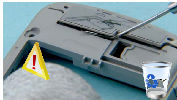
18) Carefully lift up the ANTENNA ASSY with the dental tool. The ANTENNA ASSY has always to be renewed.
