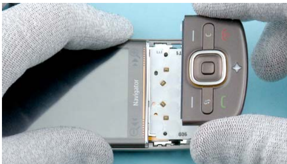
21) The FUNCTION KEYMAT can be removed.
