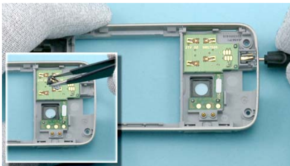
15) Use the charger plug to detach the DC jack including the light guide from C-COVER ASSY. Remove the DC jack with the tweezers.
