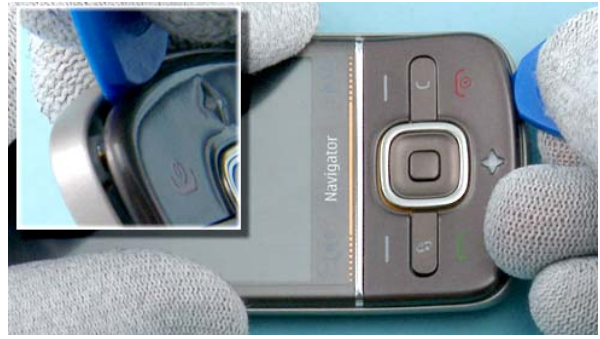
20) Use the SRT-6 to carefully lift up the FUNCTION KEYMAT. Make sure the keymat is completely detached.
