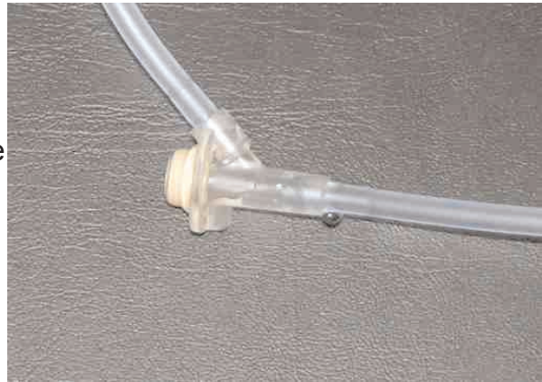
Figure 10. Drop forming outside Y-site
