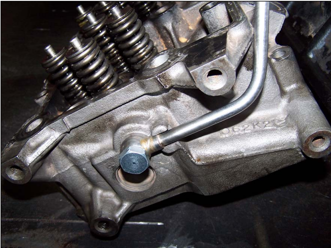
Figure 1c – Rear of Driver Side Head with Aftermarket Fuel Line
