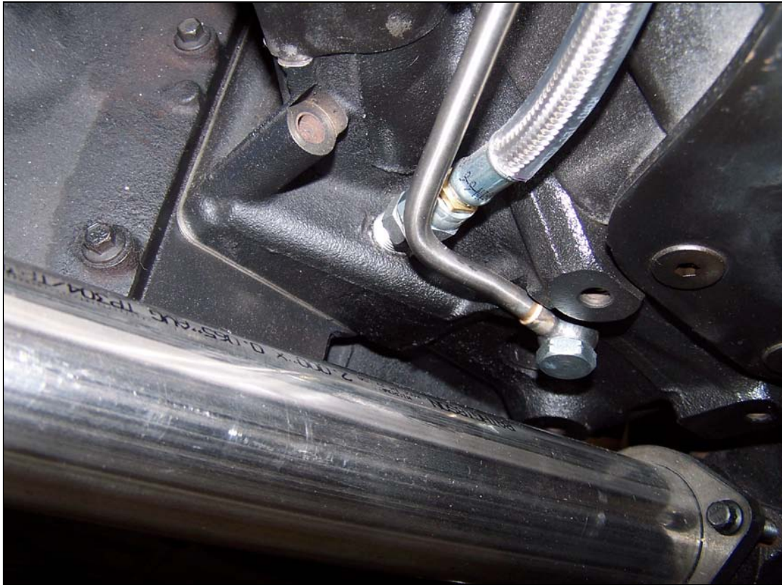
Figure 9 – Passenger Side Line In Assembled Engine (note minor bend in fuel line for clearance)
