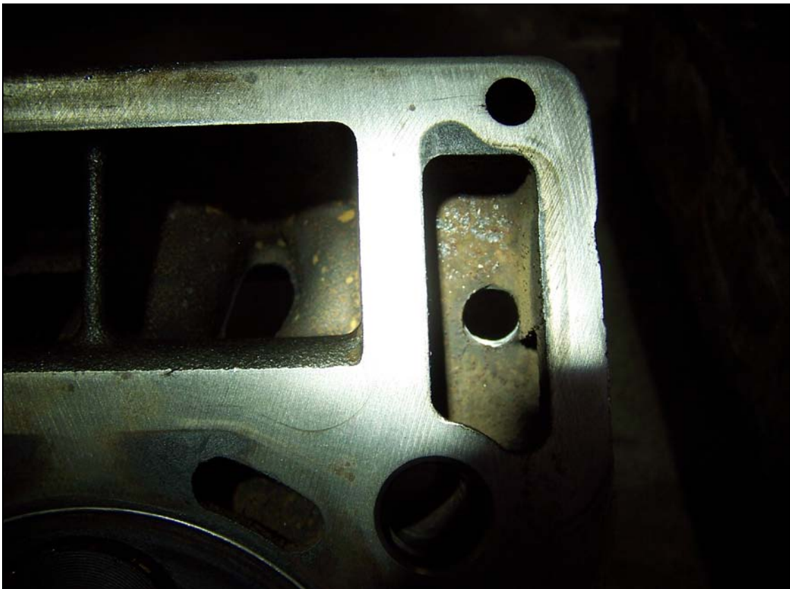
Figure 3 – Underside of Head with Hold Drilled (hole will not be centered in port)
