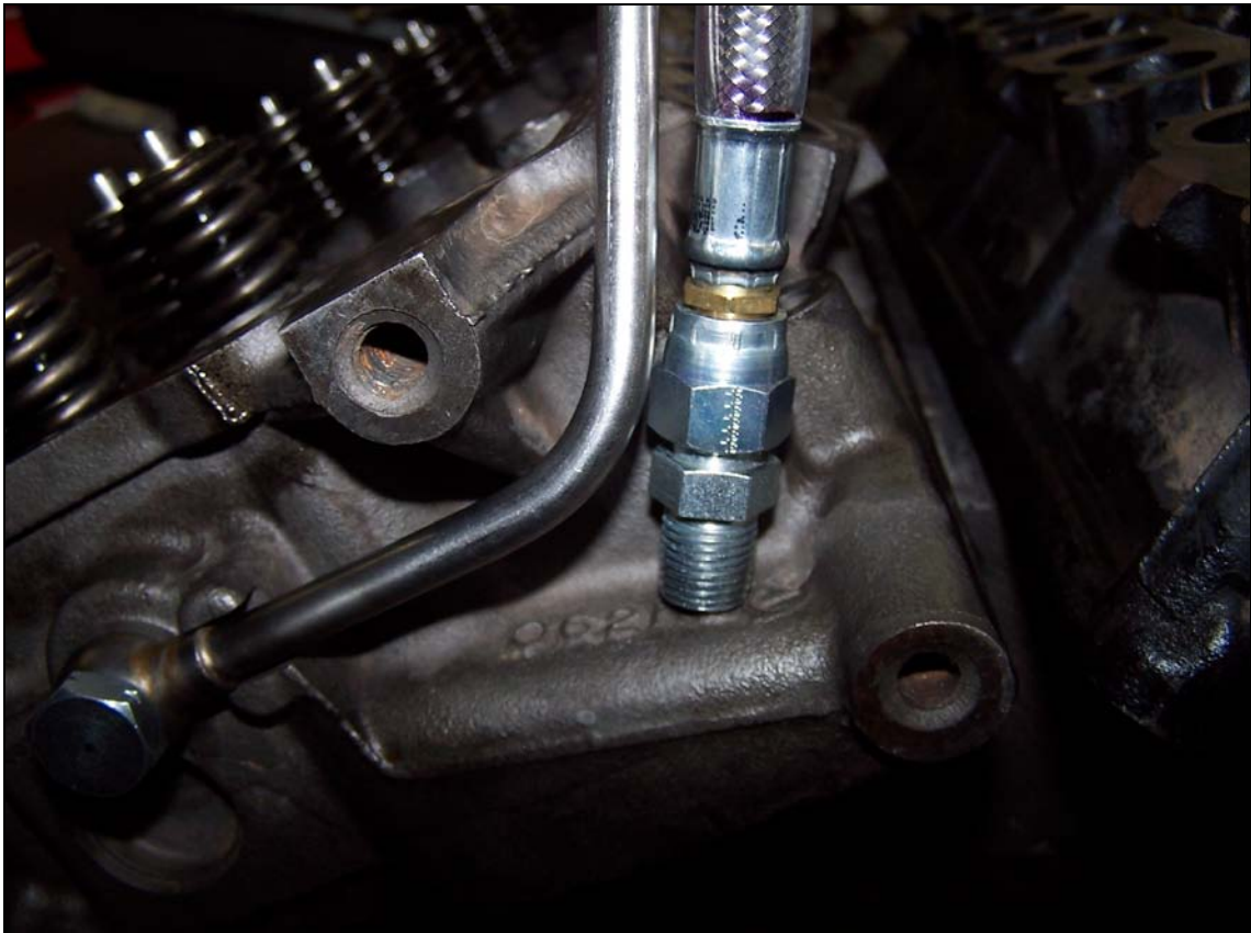
Figure 2b – Choosing Drilling Location in Driver Side Head
