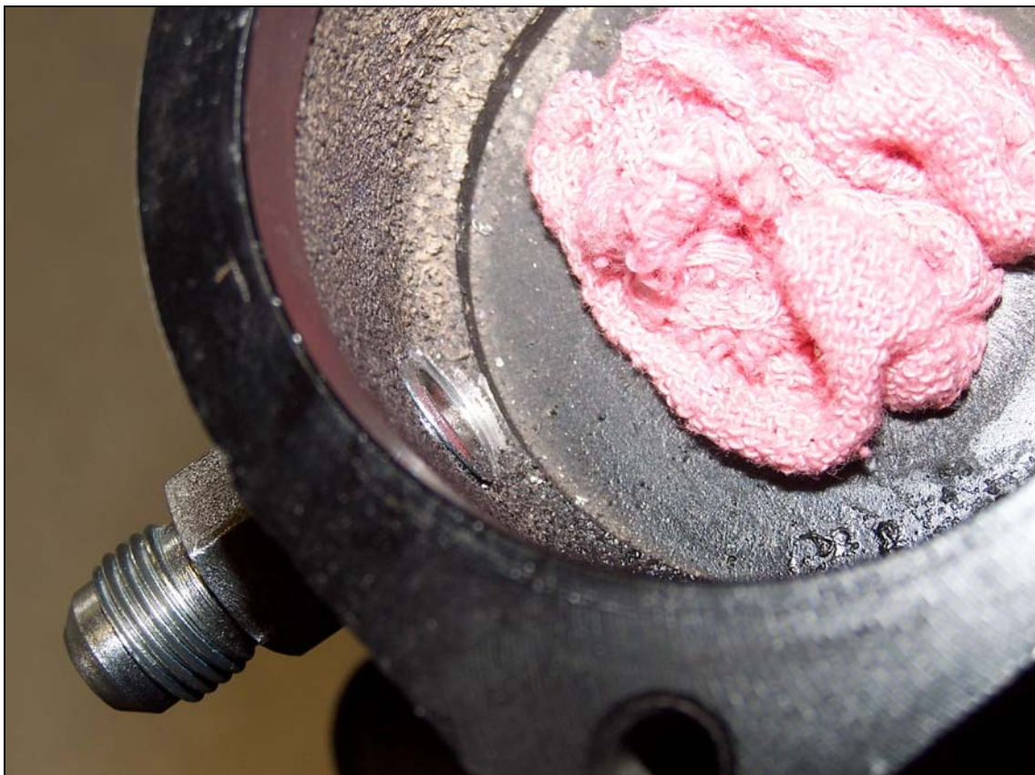
Figure 6 – Fitting Installed Flush with Inside Surface
