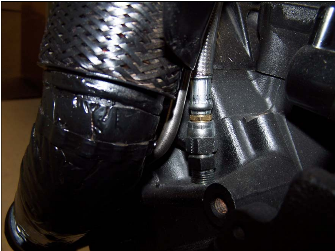
Figure 10 – Drivers Side Line In Assembled Engine
