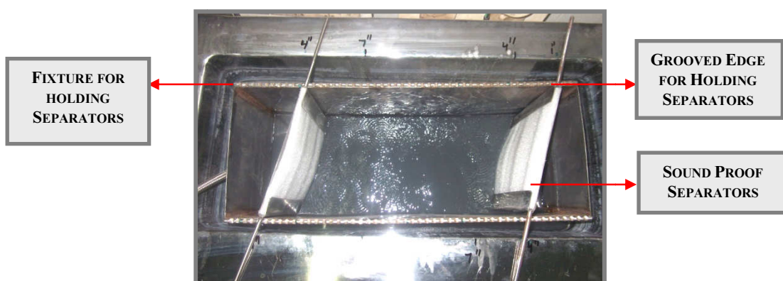
FIGURE 3.7: ISOLATION FIXTURE AND SEPARATORS IN ULTRASONIC CLEANING TANK
