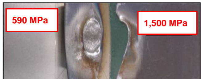
Tensile Test Results of MAG-Welded 1,500 MPa Steel
