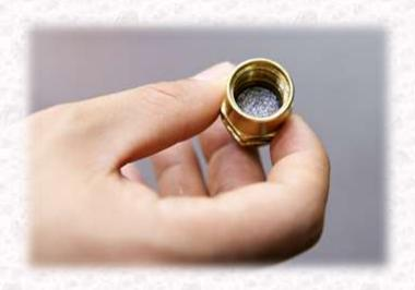
From the back end of the blade holder section (from which you have removed the blades), use a small allen key (or similar tool) to gently push the gauze free from the holder.
