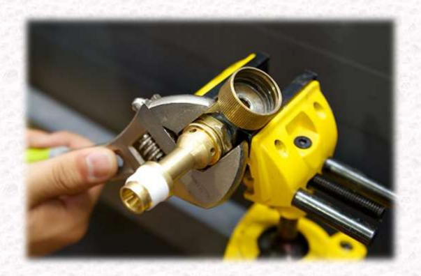
Secure the lance body in a vice (or hold firmly) and tighten the shaft onto the body using the adjustable spanner. Then reapply the O-ring you removed earlier as per the picture below.
