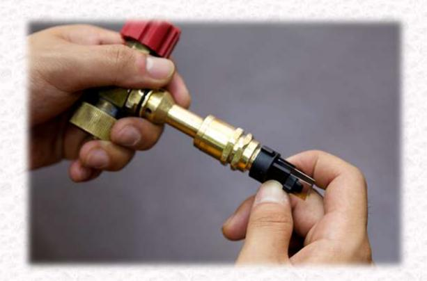
Firmly push the blades back on to the blade holder as above, leaving the partially reassembled lance looking as below, ensuring the blades are vertical.
