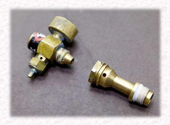
With the body now completely separate from all parts of the lance, carefully examine all holes, and ensure they are free of product. Clean using a pin, or similar thin tool.
