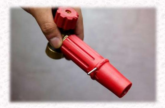
Replace the plastic part of the shaft to the lance, and replace the pin carefully into the locating hole, firmly pushing into place.
