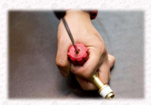
Reattach the lance adjuster to the top of the body with the screw. Apply PTFE tape to the end of the lance shaft as shown above
