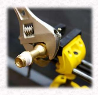
Gently loosen the lance shaft from the body at this point.
