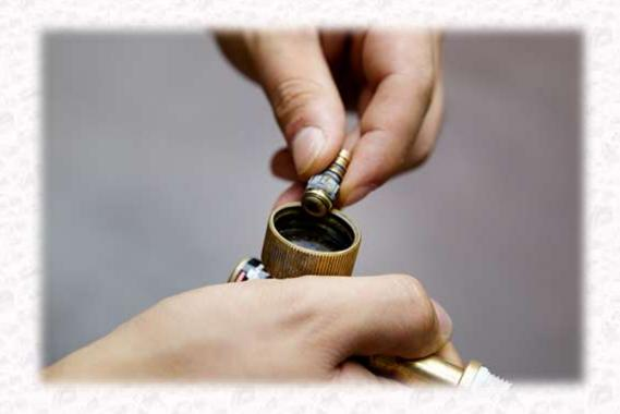
Remove the pickup inlet from the body of the lance as above. Now remove the lance shaft from the body as below.
