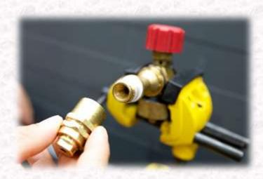
With the lance in a vice or firmly grasped, use the adjustable spanner to remove the blade holder from the lance body.
