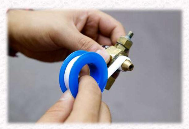
Apply PTFE (plumbers) tape to the thread as shown above, a few wraps should be sufficient. Then carefully reattach the lance shaft to the body as per the picture below.
