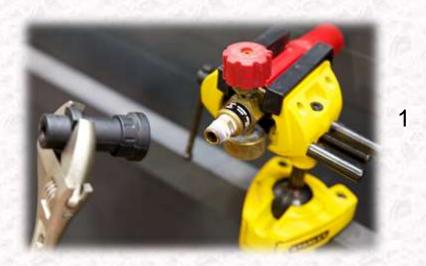
With the adaptor removed (1), carefully push the securing pin from the lance using a tool such as a small allen key (2). This will enable you to remove the plastic sheath as per the bottom picture (3).
