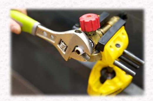
With the lance in a vice, or holding firmly, use the adjustable spanner to remove the adaptor connecting piece from the lance body, revealing the injector as per the picture below.
