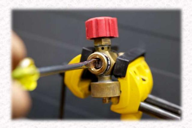
Using a flat head screwdriver, carefully turn anticlockwise the injector, removing and storing in a safe place.
