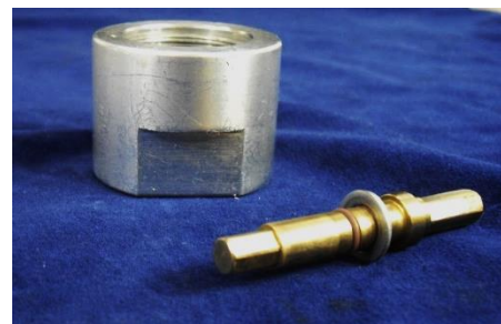
Part : 00000142-1113-000 DIFFERENTIAL ADJUSTING TOOL Used to adjust low-end differential pressure
