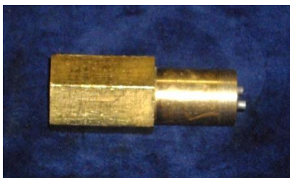
Part : 00000153-1012-000 LSH LOCK TOOL Used to install LSH Lock in Outlet Body
