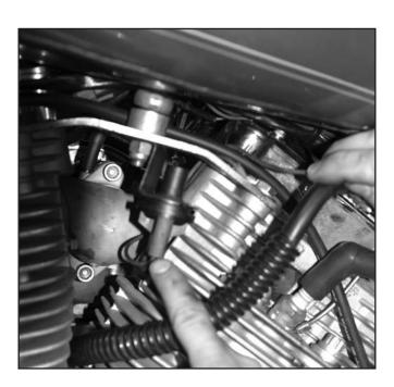
II- Connect the VOES hose from the switch to the nipple in the manifold. Trim the hose to be as short as possible without stretching or kinking it.
