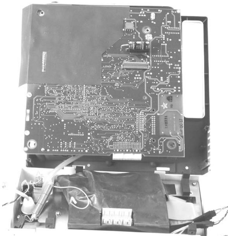
**Figure 7-5: Scholar III Open, Main Board Exposed**
