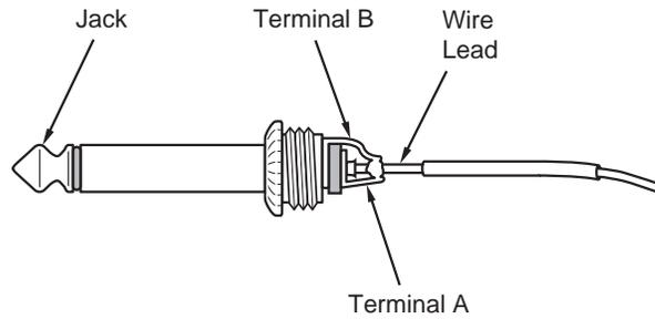
**Figure 5-2: Temperature Receptacle Test Plug**
