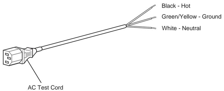
**Figure 6-2: AC Input Test Connector**
