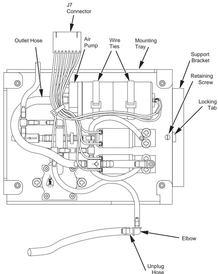
**Figure 7-10: Air Pump Installation**
