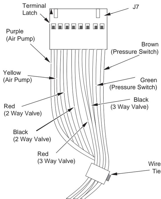
**Figure 7-11: Wire Position and Removal from J7 Connector**
