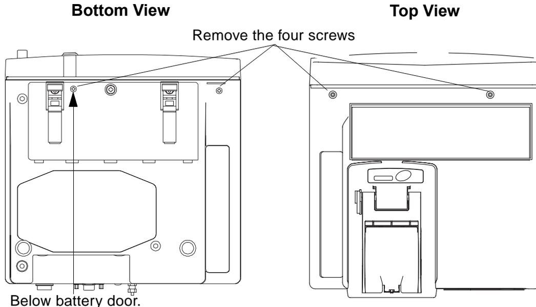
**Figure 7-13: Remove the Front Bezel**
