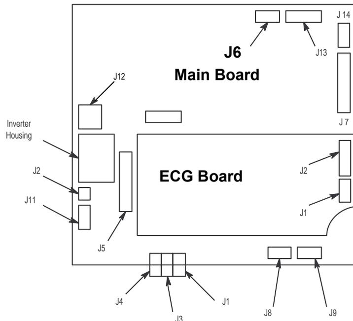
**Figure 7-4: Main Board and ECG Board Connectors**
