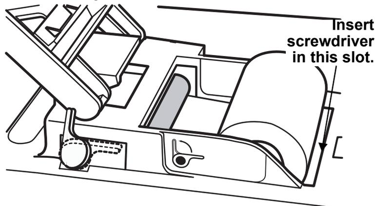
**Figure 7-3: Recorder Module Removal**
