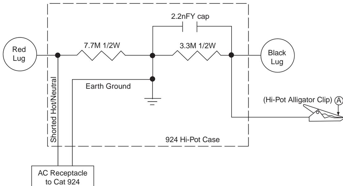
**Figure 5-1: Connecting the Y-Capacitor**
