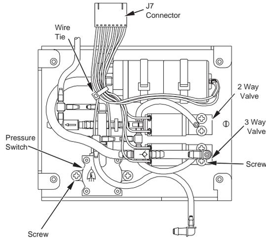
**Figure 7-12: Solenoid Valve and Pressure Switch Installation**
