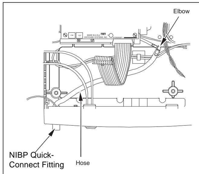
**Figure 7-14: Disconnecting Blood Pressure Cuff Hose at Elbow**
