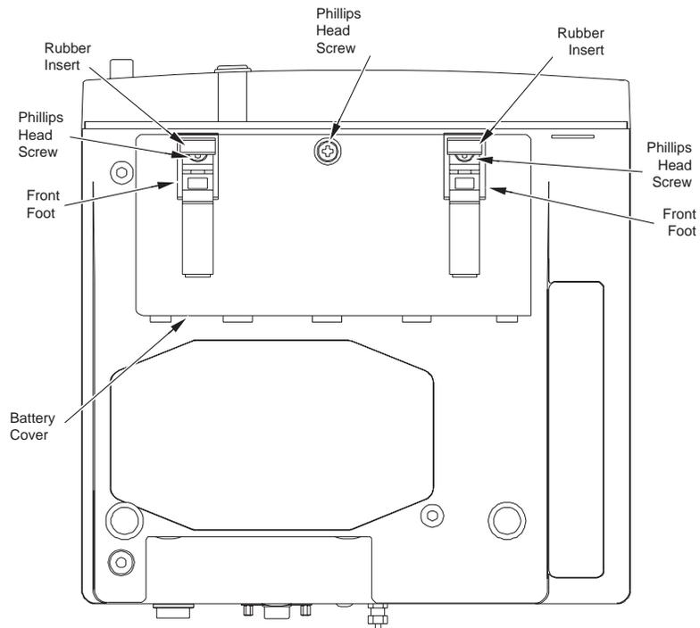
**Figure 7-1: Battery Removal**
