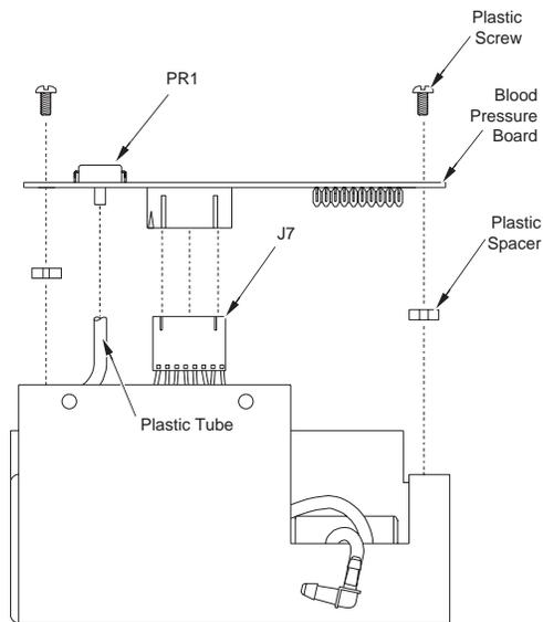
**Figure 7-9: Blood Pressure Board Replacement**
