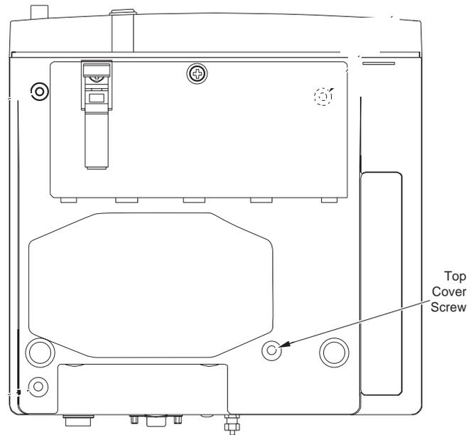
**Figure 7-6: Recorder/Printer Module Retaining Screw**
