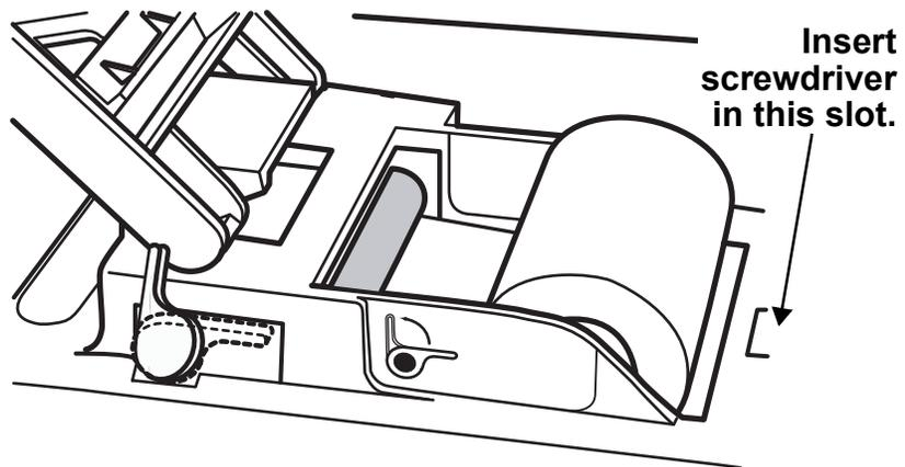
**Figure 7-7: Recorder Module Removal**
