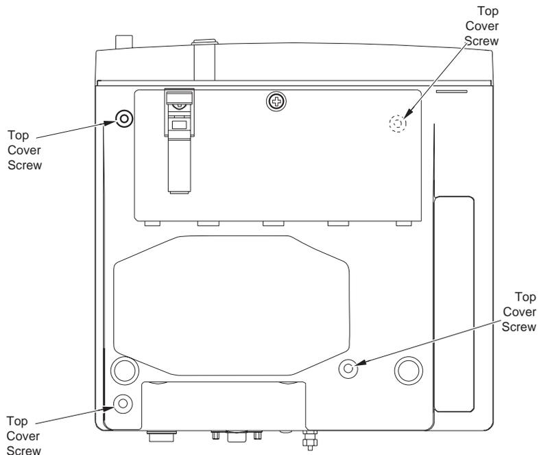
**Figure 7-2: Top Cover Removal**
