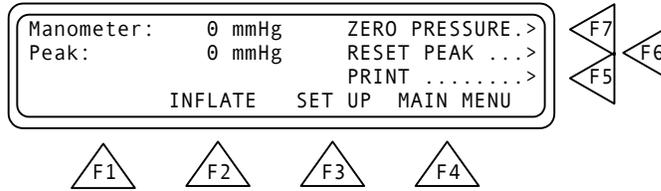
5. Press **INFLATE (F2)**. The menu changes and **DEFLATE (F2)** becomes active (*see below*). Wait until the inflation stops. When the test results are shown, press **DEFLATE**.
