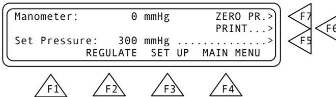
5. To reset the manometer to 0 mmHg, press **ZERO PR (F7)**.
