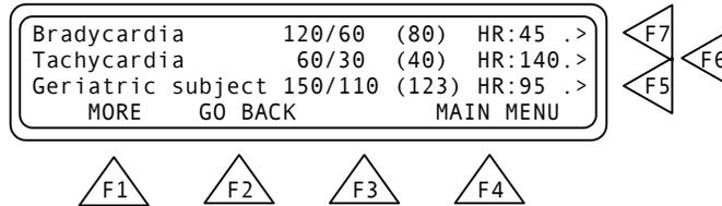
To select the desired preset use the **F5**, **F6** or **F7** key. When pressed you advance to another screen, indicating the condition's pulse pressure (PP). You also have the option at this point of selecting between adult or neonate settings for this condition. (See the Bradycardia Artifact Screen in the sequence below).
