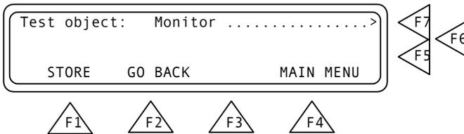
3. Press **Test object (F7)**. This allows you to select between **Monitor** and **Cuff and Monitor** as the port being used.
