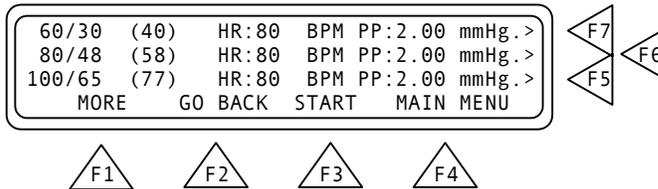
To select the desired preset use the **F5**, **F6** or **F7** key. The corresponding line will flash intermittently to indicate the selected preset. Below are the adult and neonate preset pressures.
