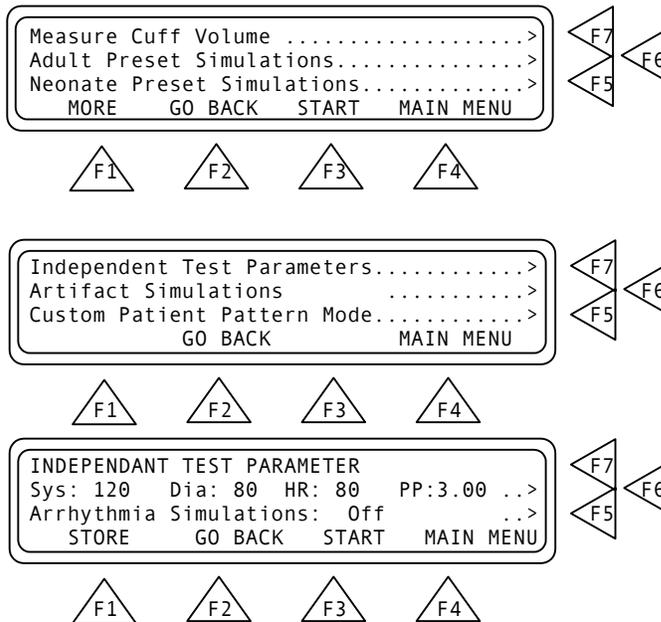
Press the **F6** key to enter the desired pressure and heart rate settings. Once **F6** is pressed a cursor appears in the setting that is to be changed. Use the alphanumeric keys to enter the following setting(s):
