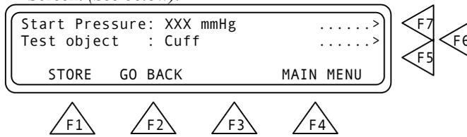
3. Use the alphanumeric keys to enter the **Start Pressure (F7)** setting to between 0 and 400 mmHg. Press the **Enter** key to save the new setting(s). Use the **Delete** key to clear the current setting.
