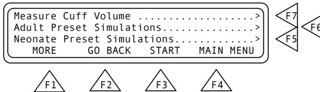
Press **START (F7)**. Pressurization of the cuff begins. The screen changes while measurement occurs (*see below*), and a new menu item, **ABORT (F3)** is added, which can be used to stop pressurization.
