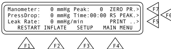
6. Press **INFLATE (F2)**. The menu changes and **DEFLATE (F2)** becomes active (*see below*). Wait until the inflation stops. When the test results are shown, press **DEFLATE**.
