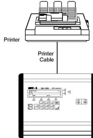
If *ansur* QA-1290 is being used, attach an RS-232C (null modem/data transfer configured) cable to the 9-pin D-sub outlet port located at the rear of the QA-1290. Do not attach the printer cable to the QA-1290. *See below.*
