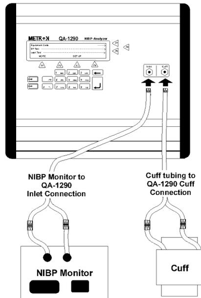
With its Tubing Kit (P.N. 17515) METRON offers a number of pressure connector adapters. The adapters connect to the QA-1290 Pressure Port via a quick-disconnect, airtight, O-ring pressure fitting. See *Appendix A, Tubing Kit Components*.
