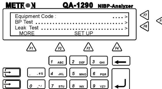
There are four text lines to each screen. The top three lines are used for operator settings, system messages, and test status and results. They are controlled by the **F5**, **F6** and **F7** keys, located to the right of the display. Note, however, that these keys are active only when you see the leading arrows ("... >") pointing to them. (See above)
