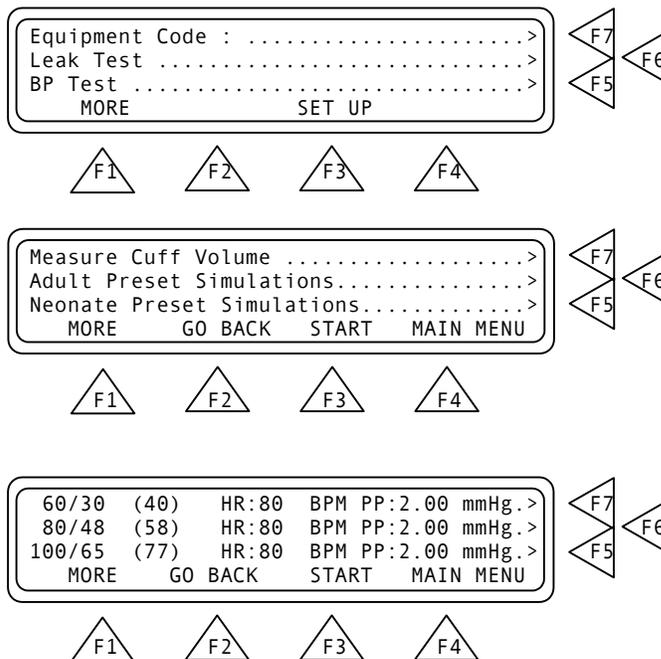
The screen changes when the test is started (*see below*). The top line of the screen specifies the settings for the test, and includes the preset diastolic/systolic pressures, mean arterial pressure (MAP), heart rate (HR), pulse pressure (PP), and what arrhythmia simulation is used (if any).
