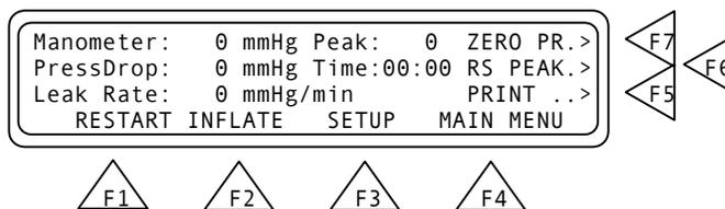
8. To repeat the test, press **RESTART (F1)**, which resets the results to zero. Then, press **INFLATE**.
