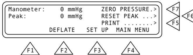
6. To reset the manometer and peak values to 0 mmHg, press **ZERO PRESSURE (F7)** and **RESET PEAK (F6)**. Note that this also resets the time to zero.
