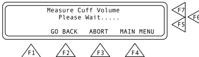
When the measurement is completed the cuff volume is displayed in cubic centimeters. Press **GO BACK (F2)** to return to the BP Test Index Screen.
