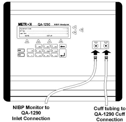
The connection of a NIBP Analyzer and cuff that use two tubes is as shown below. Tubing from the NIBP Analyzer is connected to the luer lock on the Inlet Port, while the Cuff's tubing is connected to the luer lock on the Cuff Port.
