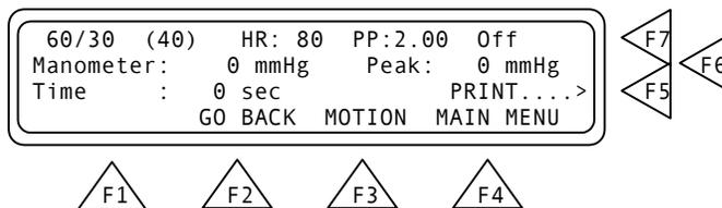
The second and third lines display test readings for the manometer and peak pressure in millimeters of mercury (mmHg), and the inflation time in seconds.
