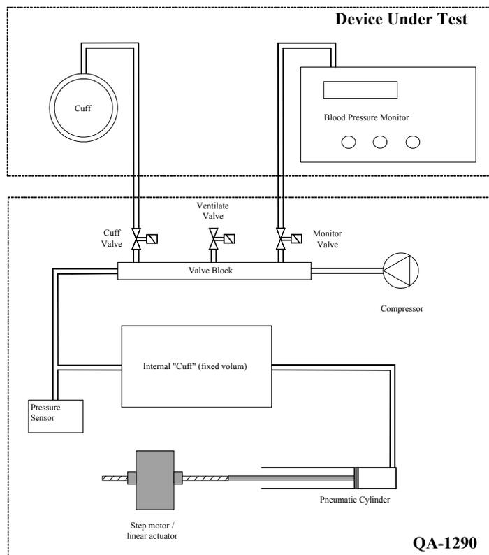
A miniature compressor generates the pressure needed for the Leak and Over-Pressure Cutoff Tests. It is also used during blood pressure simulations for creating minor, rapid increases in pressure to simulate that patient movement (i.e., when you press **MOTION (F3)**). Because the compressor may have a little leakage that affects the leak test, a back valve is inserted between the compressor and valve block.
