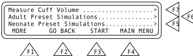
In either case you advance to a series of three screens in which you select the appropriate preset. The presets are diastolic/ systolic pressure, mean arterial pressure (MAP), heart rate (HR) and pulse pressure (PP). (*See the first screen in the sequence below*).
