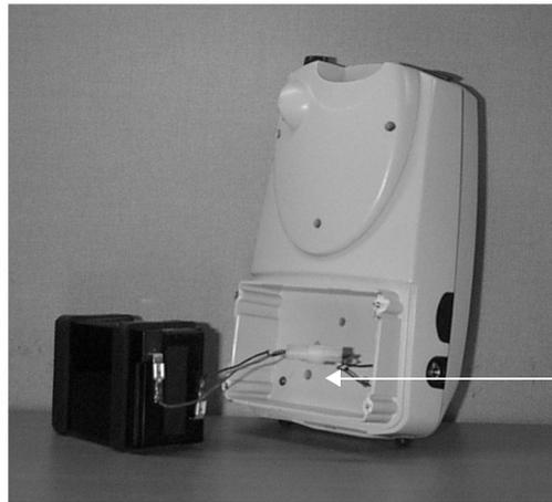
5. Slide the new battery into the battery compartment as far as it will go. Do not push the connector down into the case or lay it flat next to the battery. The relief pocket in the battery door purposely provides sufficient clearance for the battery connector.
