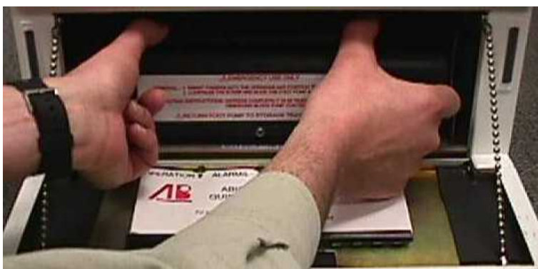
Figure 7.1 Removing the Foot Pump
