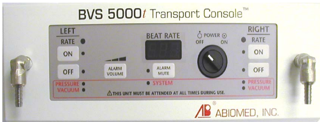
Figure 5.1 BVS 5000t Control Panel
