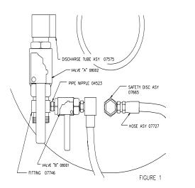
CAUTION: VALVE SHUT-OFF HANDLES MUST BE IN THE POSITIONS SHOWN WHEN EXTINGUISHER IS ON STANDBY OR IN ACTUAL OPERATION.
