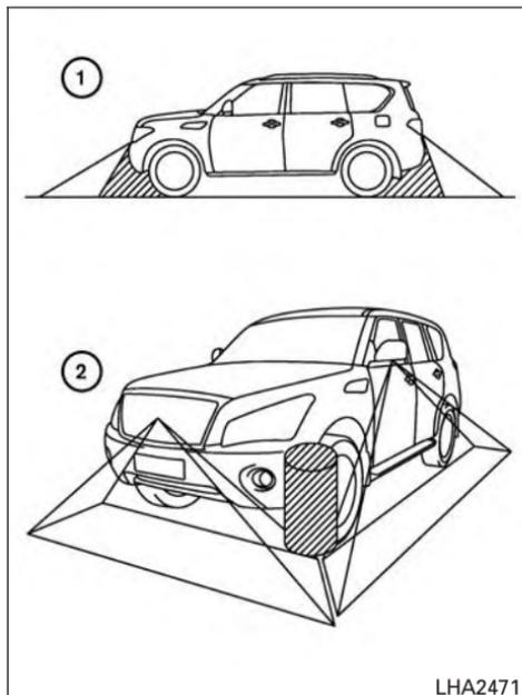
There are some areas where the system will not show objects. When in the front or rearview display, an object below the bumper or on the ground may not be viewed ①. When in the bird-eye view, a tall object near the seam of the camera viewing areas will not appear in the monitor ②.
