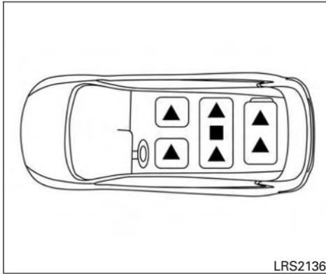
The illustration shows the seating positions equipped with head restraints. The third row head restraints do not adjust but are removable .
