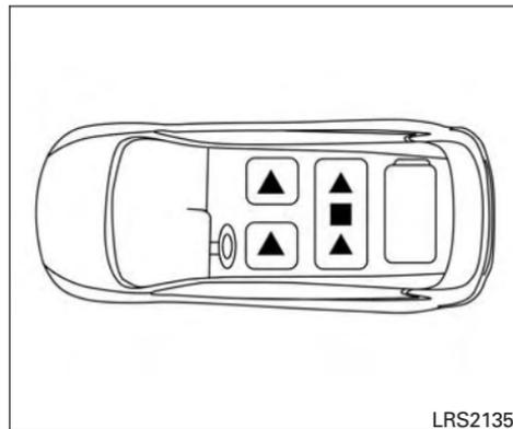
The illustration shows the seating positions equipped with head restraints. The second row head restraints are removable and adjustable.
