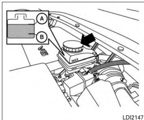
Check the fluid level in the reservoir. If the brake fluid is below the MIN line (B), the brake warning light will illuminate. Add brake fluid up to the MAX line (A). (See "RECOMMENDED FUEL/LUBRICANTS AND CAPACITIES" in the "Technical and consumer information" section for the recommended type of brake fluid.)
