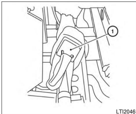
2. Locate the jumper harness connector under the lower portion of the instrument panel. The connector is taped to the wiring harness ① as indicated.
