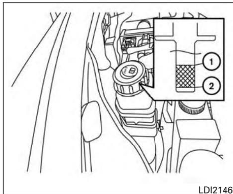
Check the fluid level in the reservoir.
