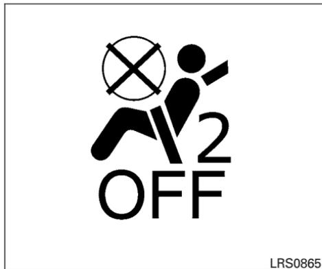
7. If the booster seat is installed in the front passenger seat, place the ignition switch in the ON position. The front passenger air bag status light
