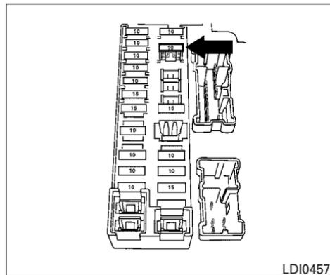
If a type A fuse is used to replace a type B fuse, the type A fuse will not be level with the fuse pocket as shown in the illustration. This will not affect the performance of the fuse. Make sure the fuse is installed in the fuse box securely.
