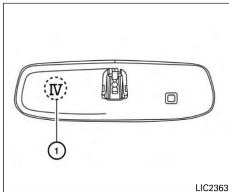
The Type B system can be identified by the IV ① on the back of the mirror. Move the mirror to see if the IV is present. If the IV is on the mirror, use the procedure in this section to program the HomeLink® Universal Transceiver. Otherwise, use the procedure in “HomeLink® universal transceiver (Type A) (if so equipped)”.
