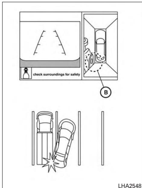
There may be a small distance visible between the vehicle and the object in the bird-eye view on the display (B). However, the vehicle may hit the object when backing up.
