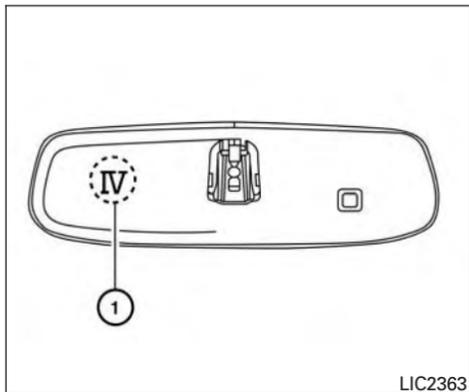
The Type A system does not have an IV ① on the back of the mirror. Move the mirror to see if the IV is present. If the IV is not on the mirror, use the procedure in this section to program the HomeLink® Universal Transceiver. If the IV is on the mirror, use the procedure in "HomeLink® universal transceiver (Type B) (if so equipped)".
