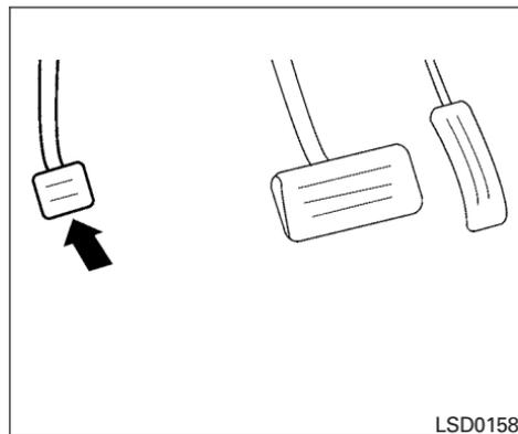
**To engage:** Firmly depress the parking brake.
