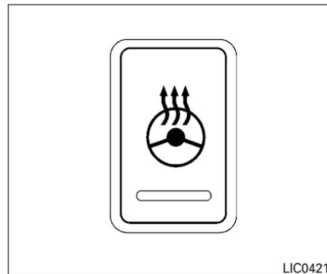
The heated steering wheel system is designed to operate only when the surface temperature of the steering wheel is below approximately 68°F (20°C).
