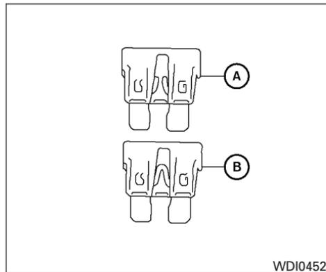
5. If the fuse is open (A), replace it with a new fuse (B).
