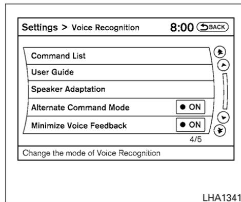
6. Alternate Command Mode is activated and the setting menu is expanded to include the Alternate Command Mode options. See “Settings menu” in this section for an explanation of the options.
