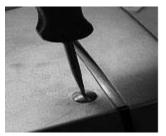
4. Each bulb socket has a release handle.
