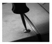
Fuse is located under the door on the PCB Remove with a small screwdriver.
