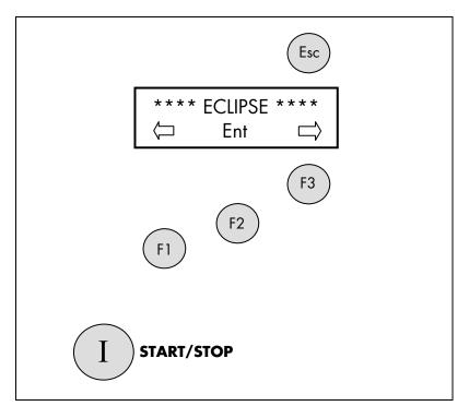
**ESC:** Changes the current display to the previous display. From Material display to accumulated Lamp time, from Program display to Material display.
