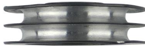
Worn Drive Pulley
