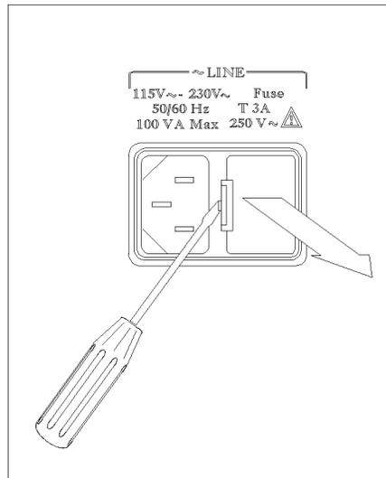
Level a small minus screwdriver to dismount the fuse holder next to the AC line receptacle on the rear panel.
