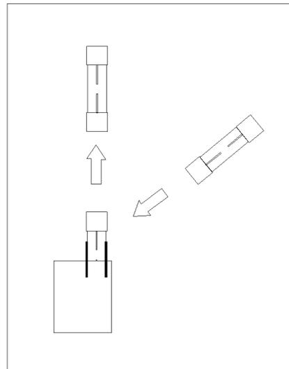
Replace the fuse in the fuse holder.
