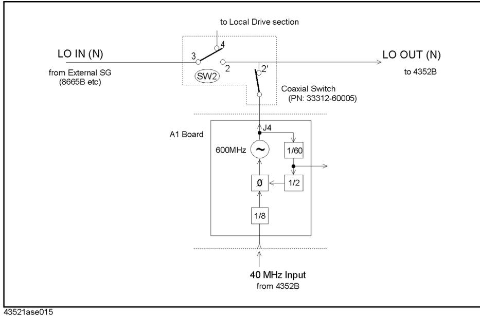
1. Turn the 43521A power off and disconnect the RF cable from the A1 connector J4. The connector location is shown in Figure 4-6.
