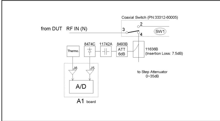
**Page 66, Figure 4-9 Heterodyne Path Simplified Block Diagram**
