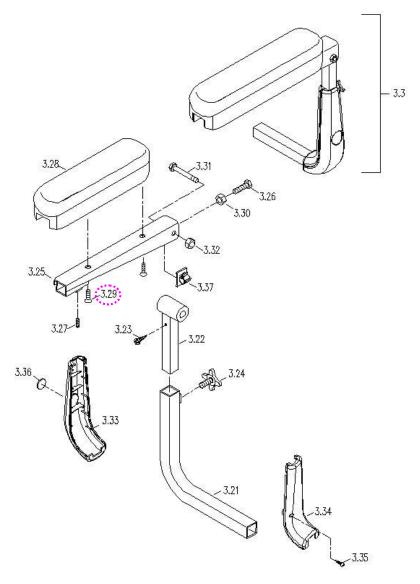
Note: The arm tube protective shrouds (3.34 and 3.35) are option parts for powerchair.
