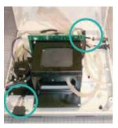
8 Before closing the housing, make sure all power leads and hoses are free from the side edges. Ensure the regulator tubing will not kink when the top cover is closed.
