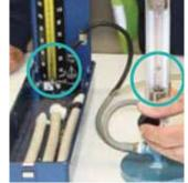
b Slowly close the valve on the Air Flow Meter to reduce airflow air and simulate 'back pressure' (i.e. to emulate the weight of a patient lying on the mattress, which forces pressure back against the flow of air from the unit). Slowly close the valve until the Sphygmomanometer pressure reading reaches 30 mmHg. At 30 mmHg, the ball bearing inside the Air Flow Meter should drop to a minimum of 3+ litres per minute.
