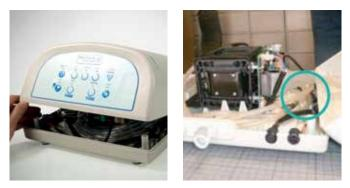
**4** Gently loosen the top and bottom housing. Once loose, hold the power socket (IEC connector) to prevent from catching while lifting the top cover and leaning it back on your work surface.
