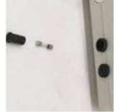
5 Insert a new fuse (or the undamaged fuse) into the plug. Push against the force of the spring and turn clockwise with the screwdriver (quarter turn).
