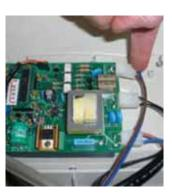
**15** Reconnect the compressor power lead to the circuit board and attach a new cable tie to secure all power leads as before.
