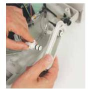
**3** Insert the replacement connector (male or female as appropriate) and turn clockwise to tighten until firm.
