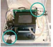
12 Before closing the housing, make sure all power leads and hoses are free from the side edges. Ensure the regulator tubing will not kink when the top cover is closed.
