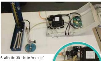
period has elapsed, detach the internal air hose from the compressor (some force may be required) and replace with the air hose from the Pressure Test Equipment (for directly connection to the compressor). Push the air hose firmly until it fully covers the connector.
