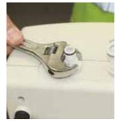
2 Using an Adjustable Wrench, unscrew the damaged quickrelease connector from the side of the unit by turning it counterclockwise – a degree of force may be required to initially loosen the connector.
