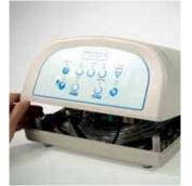
**9** Align the top and bottom housing before slowly pushing closed. Ensure the seal is properly aligned around the housing, including the air hose connectors, fuses and power socket.
