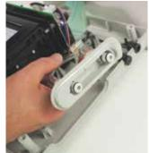
6 Detach both internal air hoses from the inside of the Connector Plate and slide the damaged plate from the side of the unit. Dispose of the Connector Plate in an environmentally safe manner.
