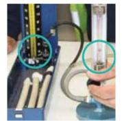
c Continue to increase back pressure resistance. Slowly close the valve on the Air Flow Meter until the Sphygmomanometer pressure reading reaches 60 mmHg. At 60 mmHg, the ball bearing inside the Air Flow Meter should drop to a minimum of 2+ litres per minute.
