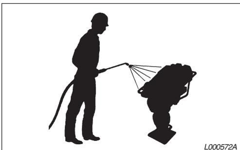
5. Keep machine clean. The machine shall always be upright when washed.
