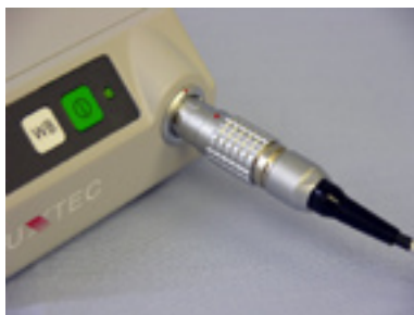
Step 4: Camera head connection via camera cable
