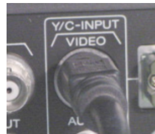
S-Video cable connected to the Y/C INPUT (S-video connection)
