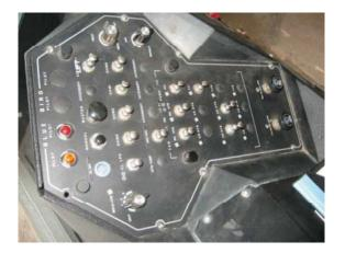
3f) Set lights for your walk-around – turn on headlight low beams, marker/clip lights, sign light, master flasher switch, and left turn signal.
