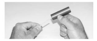
Hold the screen up to the light and look through it to make sure it is clean. All openings in the mesh should be clear. If any of the openings are blocked, clear them by blowing air through the screen. If the screen cannot be 100% cleaned, replace it with a new one. A new screen is included with each new wick.
