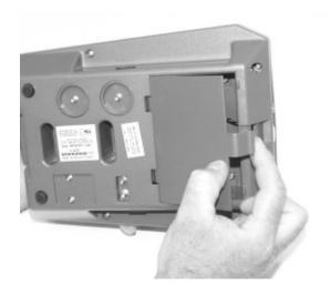
2. Locate a fully charged battery pack and plug it into the battery connector located inside the battery compartment. Note that the two connector pins are different sizes. Make certain that the connector is inserted into the battery pack with the correct polarity. DO **NOT** force the connector into the battery pack. It should slide in easily. If it does not slide in with little effort, you probably have the pins reversed.
