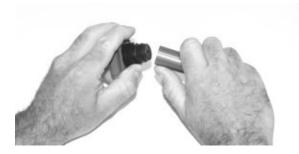
After separating the two halves, push the Alcohol Wick and screen out of the Wick Retainer Cap from the opposite end with the Wick Removal Tool (wood dowel) provided with each new alcohol wick. Do *not* use a pencil point because bits of lead could break off. Allow the small, circular, fine-mesh screen to fall out on the table.
