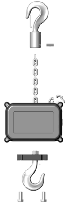
Figure 5: End view of a single-fall EXE-Rise hoist
