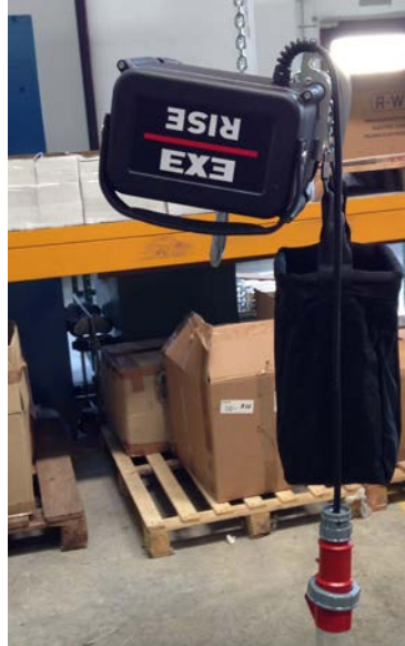
Figure 18: The hoist mounting in self-climbing mode.
