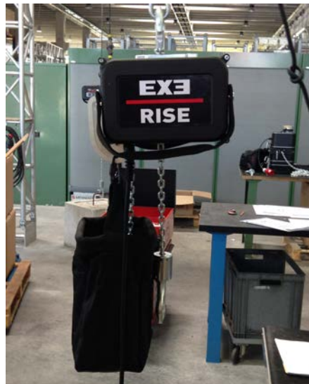
Figure 19: Mounting the hoist “body-up”
