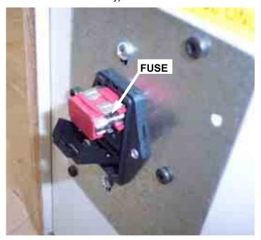
Three fuses are located on the Power Supply PC Board, and one fuse is located on the AC Power PC Board. Using a small flat blade screwdriver, pry the fuse from the fuse holder. Remove the fuse from the fuse holder and test each fuse as required. the fuses. Be sure to replace the fuses with the same type and value.
