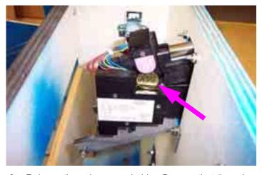
6. Release the coin sensor holder. Be sure that the coin or token is properly seated.
