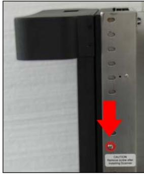
5. Remove five (5) screws from the top end cap, then gently lift the top end cap away from the wall or cart mount.
