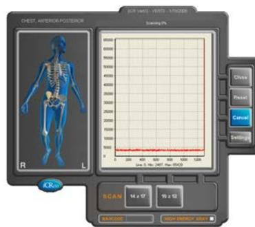
7. Open the dust cover of the iDR, the Data line should rise and lower slightly according to the position of the bay door. If the room is illuminated by high frequency fluorescent lights, the line may become sinusoidal (Wavy) and move away from the zero point.
