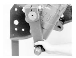
Check for sector shaft lash 3. From the "center of travel" position, grasp the pitman arm and gently try to rotate it back and forth. If looseness or lash is felt at this point, the sector shaft is out of adjustment.
