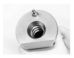
Inspect rack piston and worm ball track grooves
