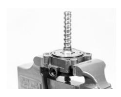
Place valve housing and valve assembly in vise 1. With worm vertical, place the valve housing, input shaft, valve/worm assembly in a vise.
