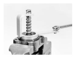
Remove bearing adjuster locknut
