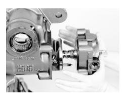
Install rack piston, worm, valve assembly
