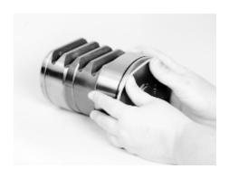
Install rack piston o-ring and seal ring 8. Install a new backup o-ring (21) and then a new Teflon seal ring (20) on rack piston (19). Do not over-stretch these rings as you install them. Do not allow the Teflon seal ring to be twisted.
