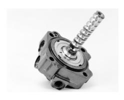
Inspect input shaft, valve/worm assembly sealing areas
