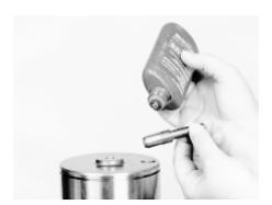
Apply Locquic "T" primer and Loctite RC680
