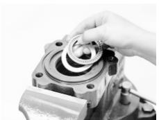
Remove thick washer and bearing
