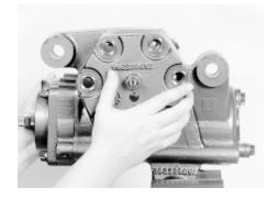
Install sector shaft and side cover into housing
