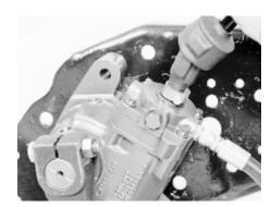
Center the sector shaft 1. With the engine on, rotate the steering wheel (input shaft) until the timing mark on the sector shaft lines up with the mark on the housing. The line on the sector shaft should be at a 90° angle from the input shaft. The sector shaft is now on its "center of travel". Turn the vehicle off.
