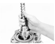
Assemble input shaft, valve worm & bearing assembly
