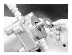
Remove dirt & water seal
