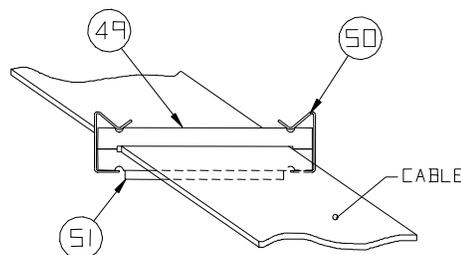
11. Remove the protective paper from the tape on the attenuator and adhere the attenuator assembly with the ribbon cable to the top of the card cage.
