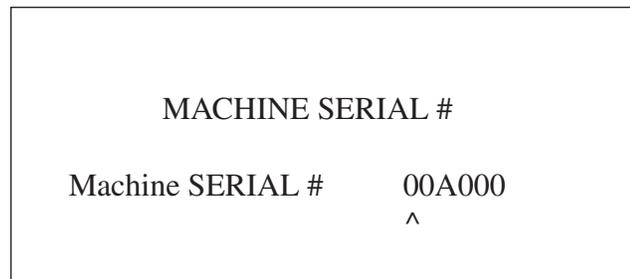
5. Use the “YES” and “NO” keys to change the digit or character selected, as indicated by the “^” cursor. Use the “MODIFY” key to advance the cursor to the next digit/character. Change all digits or characters until the display serial number matches the machine serial.
