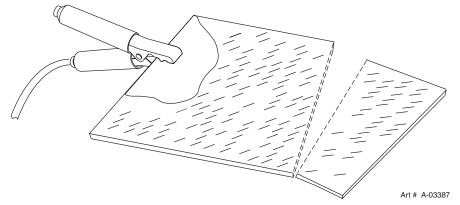
Figure 4-4 - Work Cable Connection
