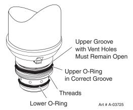
Figure 6T-1 - Torch Head O-Ring
