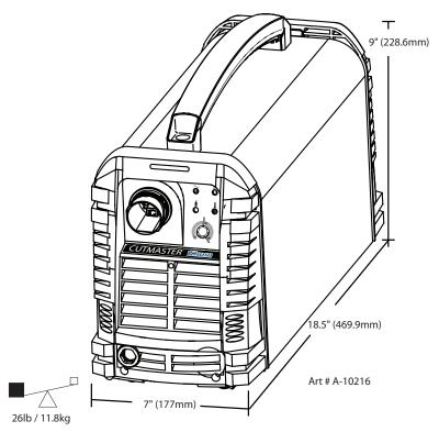
Figure 3-3 - Power Source Dimensions & Weight
