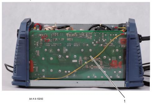
Figure 6-3 Clear Protective Sheet Removal View
