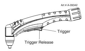
Figure 4-10 - Torch Trigger Release
