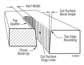
Figure 4-12 - Cut Quality Characteristics
