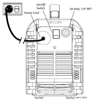
Figure 4-5 - Rear Panel with ON/OFF Switch
