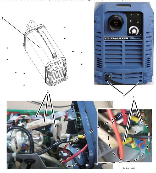
Figure 7-2 Removing Front Panel Assembly
