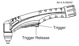
Figure 4-7 Torch Trigger Release
