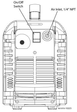
Figure 3-1 - Gas Connection to Compressed Air Input
