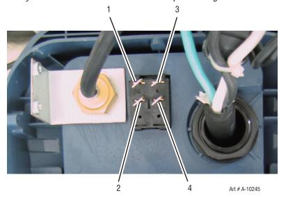
Figure 6-5 Main ON/ OFF Switch View
