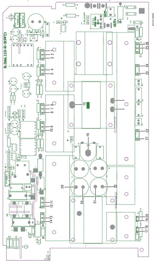
Figure 6-4 Main Inverter Board
