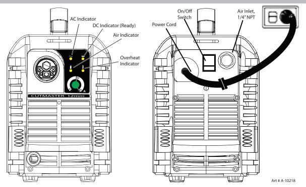
Figure 4-1 - Front Control Panel
