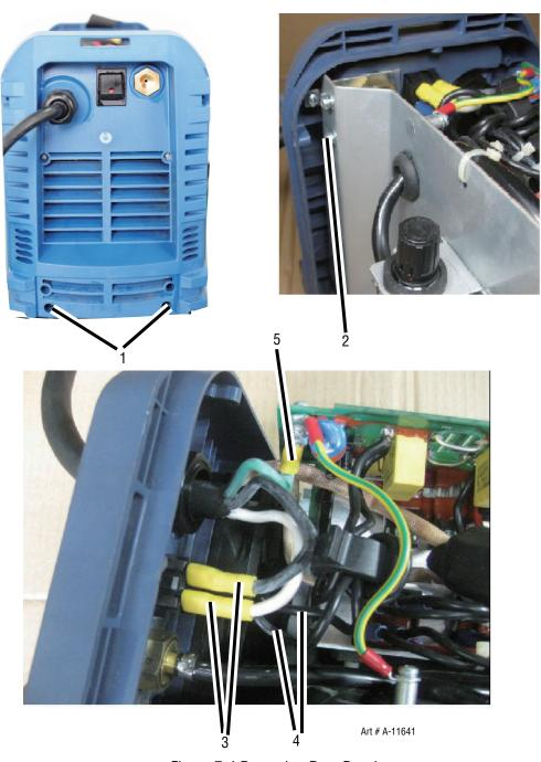
Figure 7-4 Removing Rear Panel
