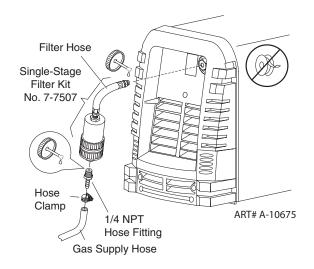
Figure 3-2 - Optional Single - Stage Filter Installation for Compressed Air Input
