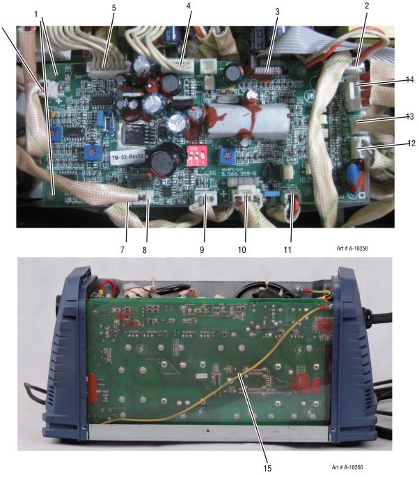
Figure 8-4 Installing Main Control PCB and Clear Cover Sheet
