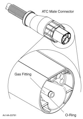
Figure 6T-2 - ATC O-Ring
