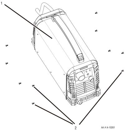
Figure 8-5 Installing the Case
