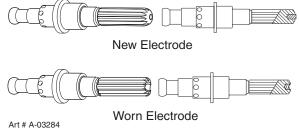
Figure 6T-6 - Electrode Wear
