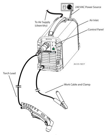
Figure 2-2- Power Supply Features
