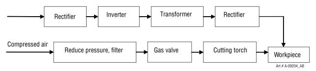
Figure 2-1- Working Principle
