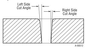
Figure 4-13 - Side Characteristics of Cut
