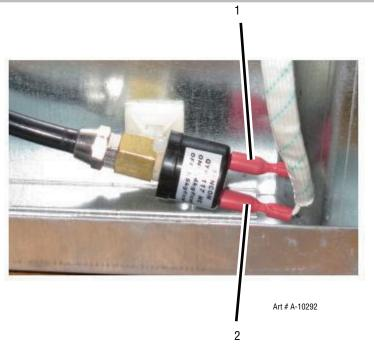
Figure 6-6 Pressure Switch View
