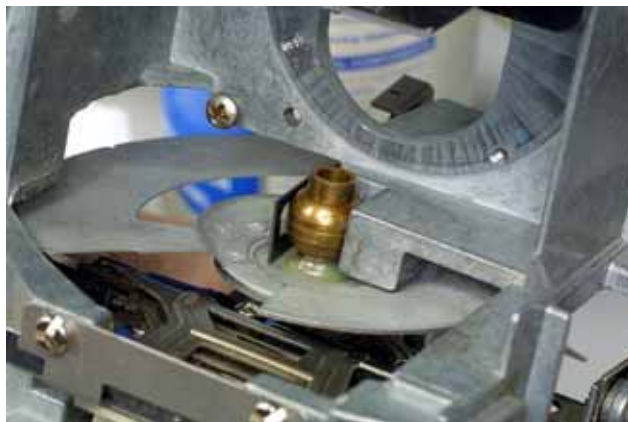
FIG. D65 Seat the shutter-side bearing. Here we've flipped an early style shutter-side bearing so the large surface faces the new-style shutter.
