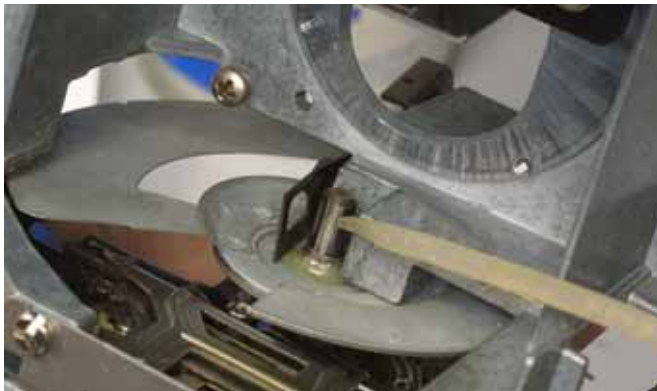
FIG. D64 Lubricate the front of the shutter-drive shaft with shutter oil.
