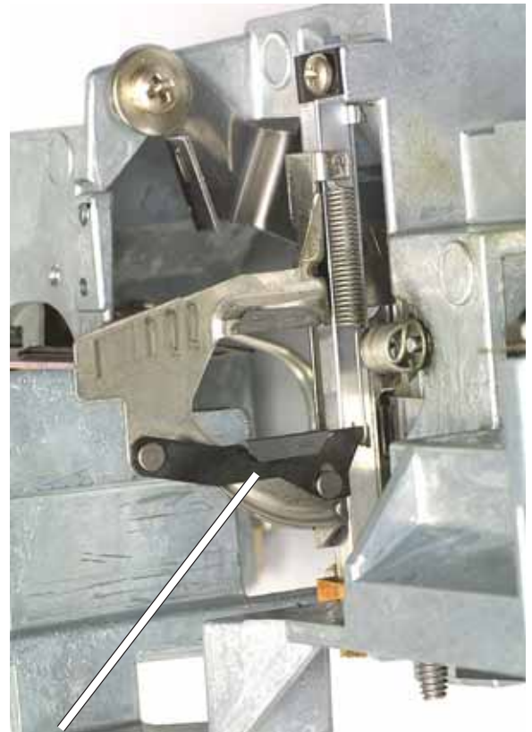
FIG. D61 Installation position for the M80 shutter-drive shaft—start with the large lobe on the dashed line and then turn the shutter-drive shaft clockwise to the position shown.
