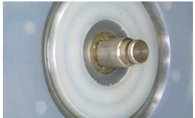
FIG. D71 Variation—this is the center of the in-and-out cam in the M85, a single-speed projector. Use the two-shoulder bushing as it's supplied. No modification is necessary.
