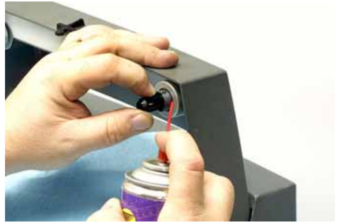
FIG. D119 Cleaning the supply spindle.
