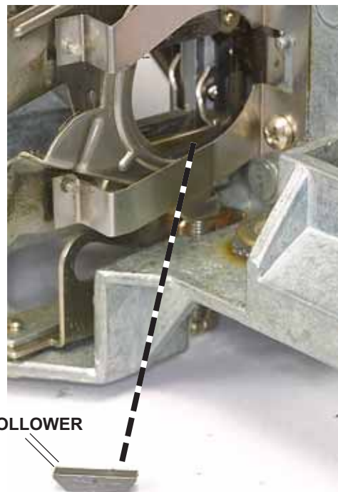
FIG. D52 Cam follower removed from the claw assembly. The cams on the shutter-drive shaft ride against this follower to provide the up-and-down claw movement.
