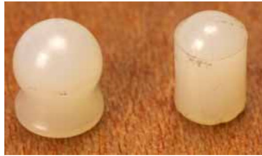
FIG. D123 A projector that runs only super 8 uses the knob-like follower on the left. A projector that runs both super-8 film and regular-8 film uses two of the bullet-shaped followers on the right. Both types come in different lengths for adjustment.
