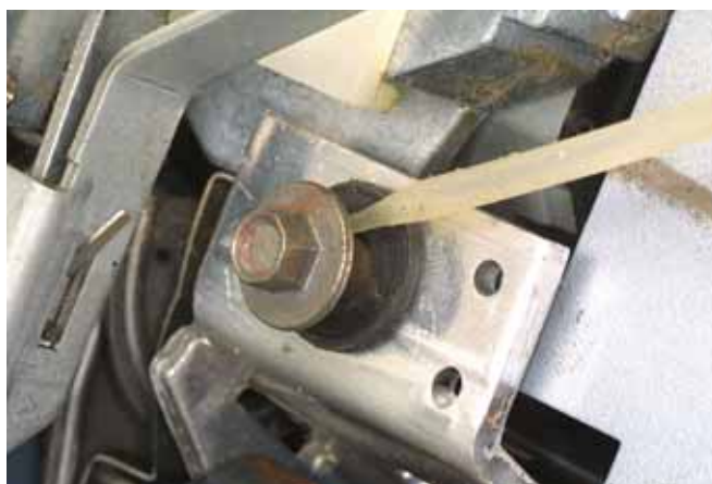
FIG. D102 Oil the grommet or the screw; the oil prevents the rubber grommet from turning as you tighten the screw.
