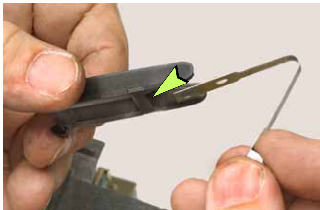
FIG. D90 Installing the spring/roller unit in the new damping arm.
