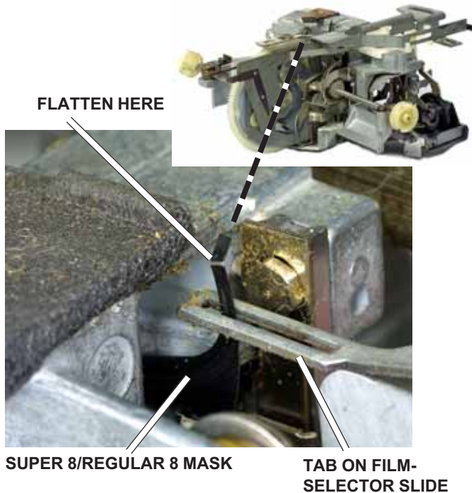
FIG. D40 Coupling to the super-8/regular-8 mask.
