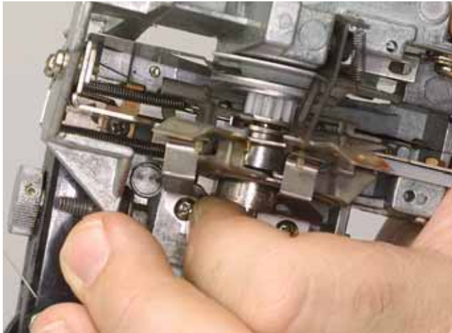
FIG. D62 Holding the shutter-drive shaft in place to replace the parts at the front of the shutter.
