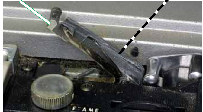
FIG. D2 A broken damping arm.
