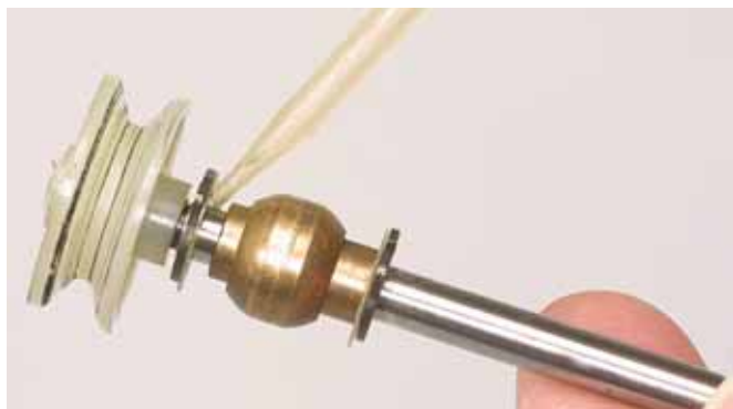
FIG. D59 Lubricating the shutter-drive shaft.
