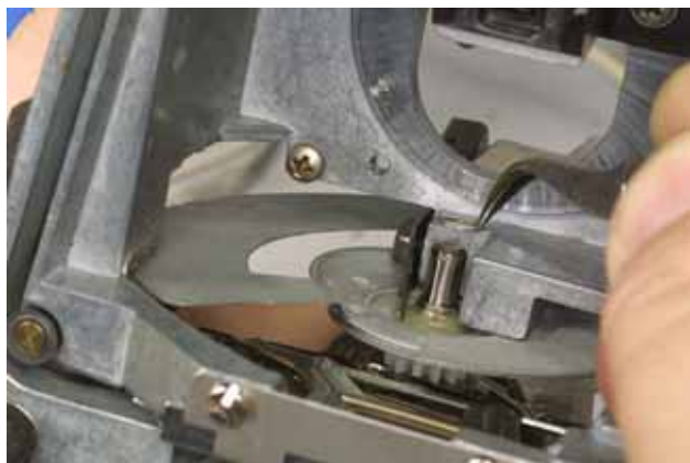
FIG. D64 Replacing the washer over the shutter-drive shaft.
