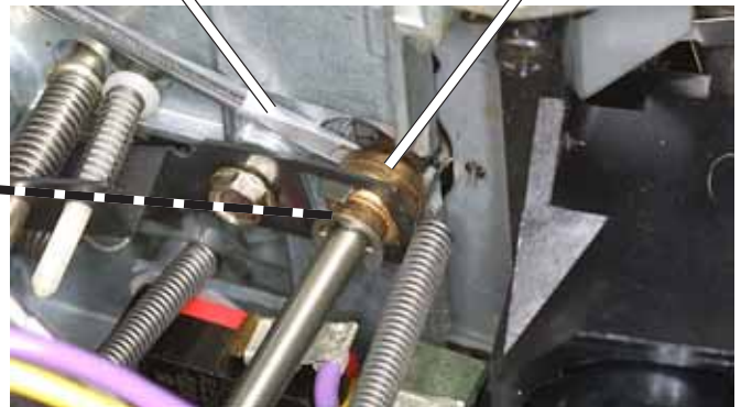
FIG. MD18 Using a screwdriver to free the shutter-drive shaft.
