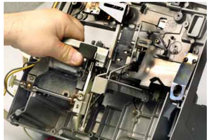
FIG. D33 Lifting the mechanism from the case.
