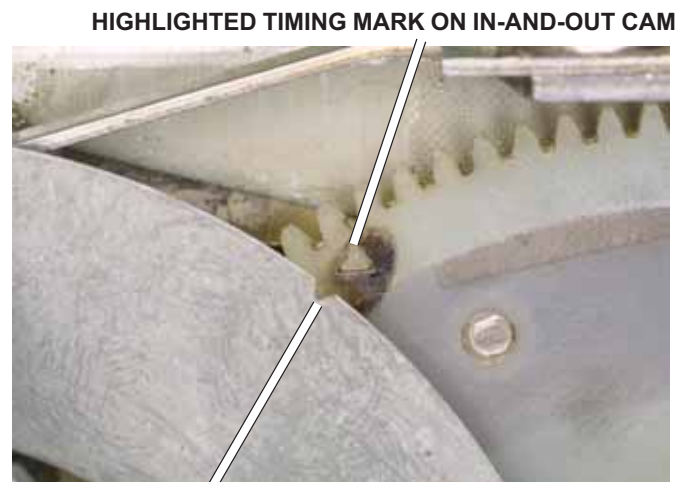
FIG. D82 Here the shutter and the in-and-out cam are properly timed.
