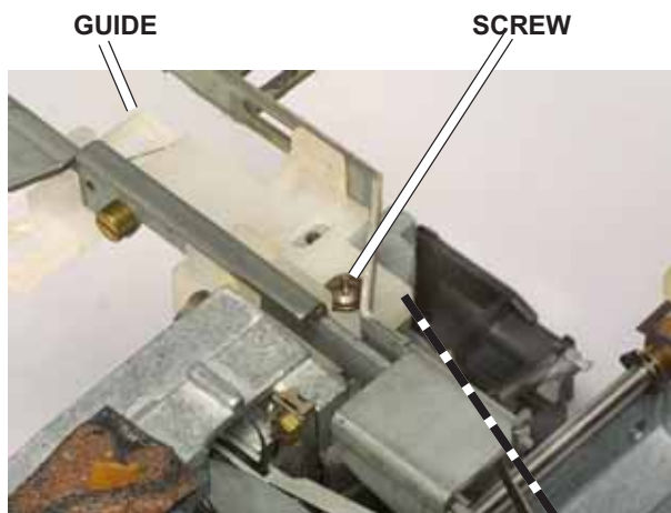
FIG. D98 Top of the mechanism, viewed from the back. Here we've replaced one screw to hold the guide.
