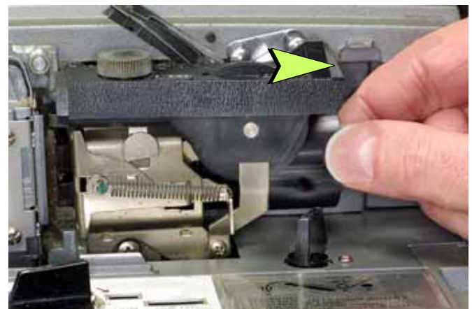
FIG. D13 Front view, front cover removed—removing the lens.
