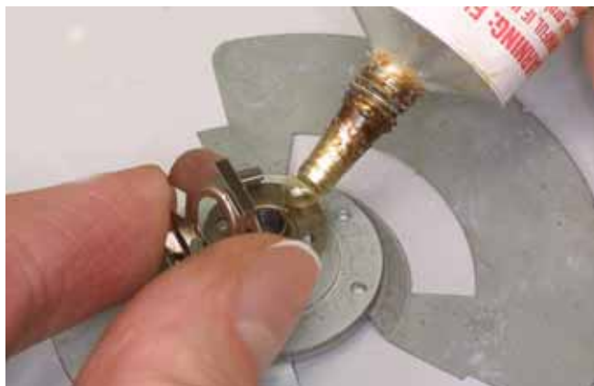
FIG. D58 You can cement the spring unit to the front of the shutter using Pliobond.
