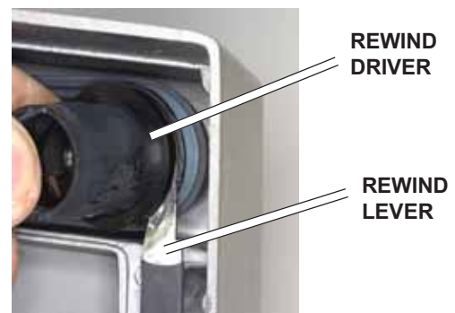
FIG. D114 Tilt the rewind driver to clear the rewind lever.
