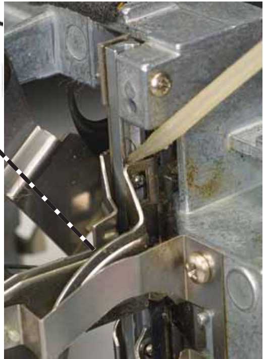
FIG. D54 Use the shutter oil to lubricate the ball bearings in the claw assembly.
