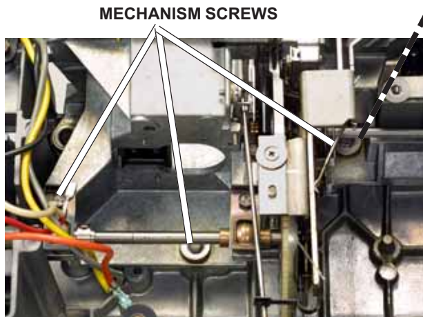
FIG. D32 Remove the three mechanism screws.
