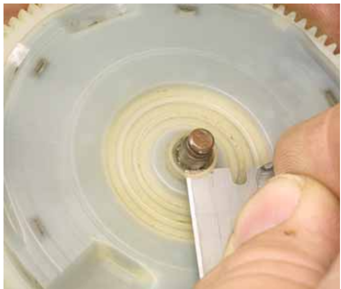
FIG. D76 Modifying the in-and-out cam by cutting back the shoulder to the groove.
