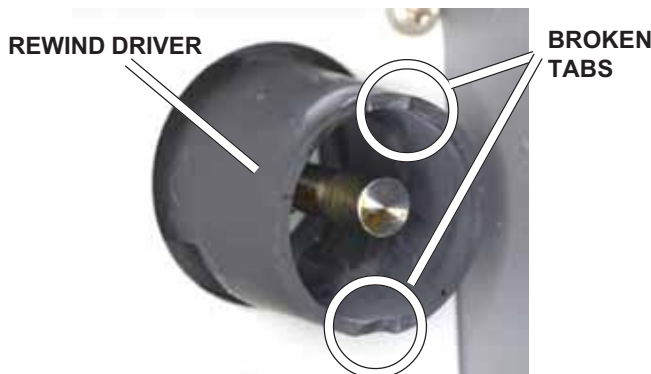
FIG. D110 Here's the typical rewind problem—the tabs are broken off the rewind driver.
