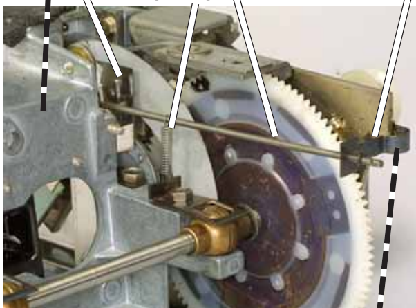
FIG. D95 Still-frame changeover rod installed in the mechanism.
