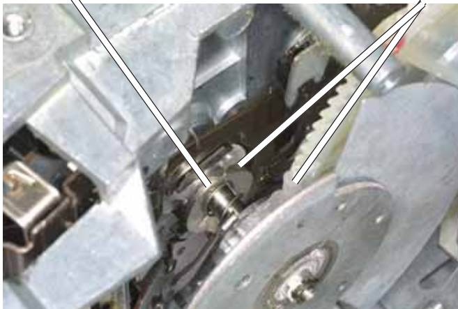
FIG. MD22 Grease lubrication points.
