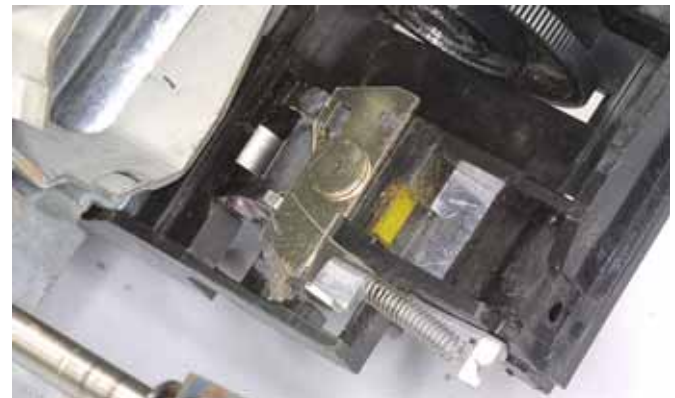
FIG. D96 Variation in the latching mechanism for the damping arm. Here the spring does not disconnect when you remove the damping arm.
