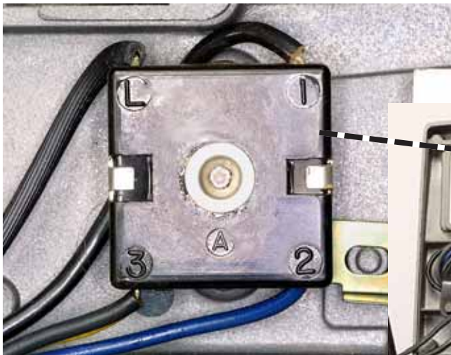
FIG. D8 Variation —the switch position is slightly different in the M90 and M95 projectors. The L port is in the upper left-hand corner.
