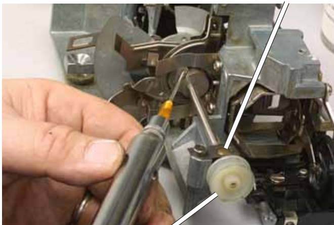
FIG. D66 Lubricate the cams of the shutter-drive shaft with grease.
