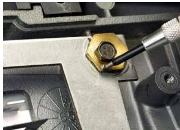
FIG. D15 Scribing the eccentric bearing for the forward/reverse arm.
