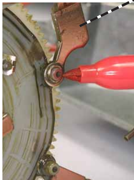
FIG. D43 Marking the super-8 follower with a felt-tip pen.
