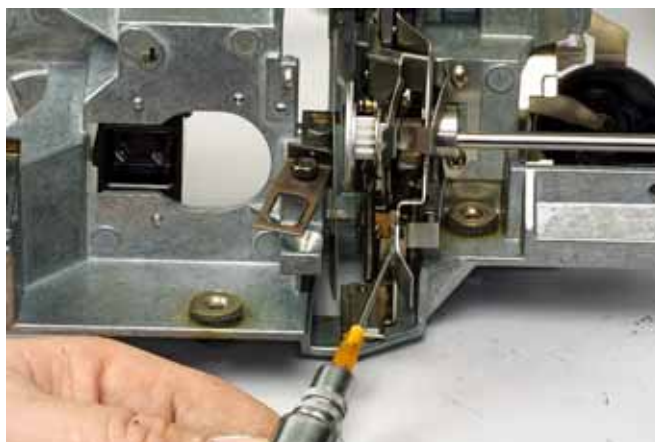
FIG. D68 Lubricate the arms that contact the in-and-out-cam followers with grease.
