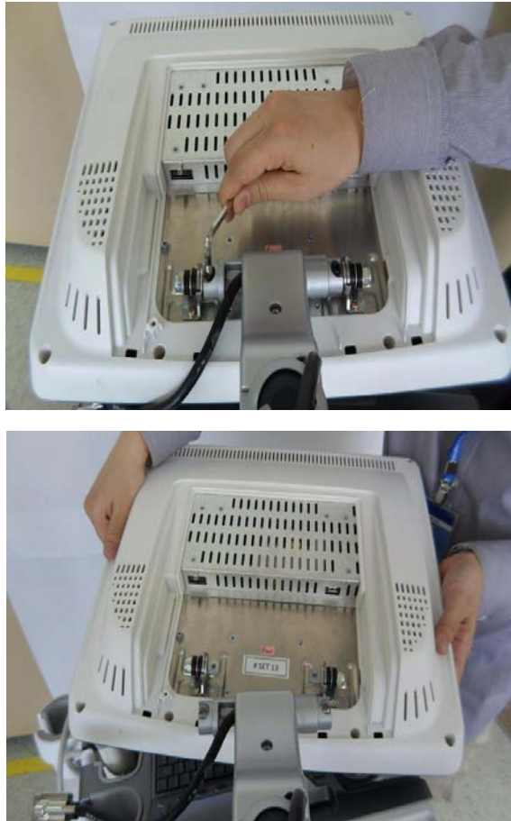
Figure 8-22 Unscrewing 2 screws & separating the Monitor
