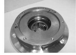
Separate the lateral reduction unit from the axle and place it on a flat surface.
