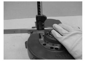
Temporarily position the tapered roller bearing (4) in its cup and measure value "B" as illustrated in the figure using a depth gauge.
