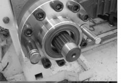
Position the shim ring (23) on the brake lever's pin (17).
