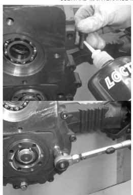
Tighten the screws (2) with washer (3) applying Loctite 270.
