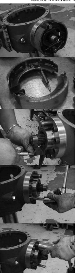
Remove the 2 brake shoes (20) with the 2 contrast springs (21) from the pin seat (19) and from the brake lever (24).
