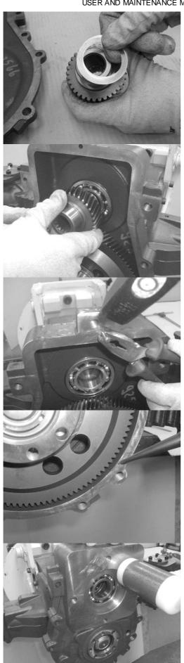
Position the shims (8) on the driving gear (7) by the shoulder opposite the grooved profile.
