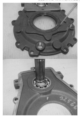
Remove the sealing ring (1) from the cover with a screwdriver.
