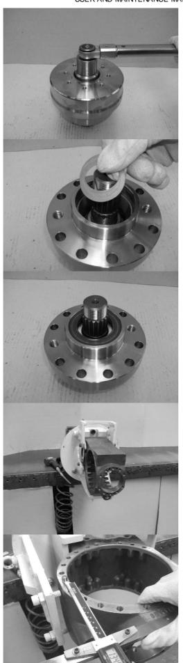
Check the pre-load value of the tapered roller bearings (4) and (10) measured as the rolling torque with a torquemeter.
