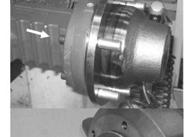
Remove the securing screws and washers fixing the wheel reduction unit to the lateral beam.
