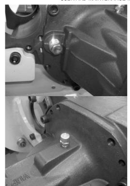
Tighten the closing plug (6) at a torque of 3 daNm.
