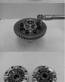
Undo the securing screws (8) of the bevel crown (9) from the differential housing and separate the crown.
