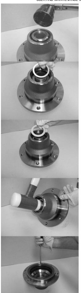
Unscrew and remove the M50x1.5 ring nut (21) with the commercial tool (T04).
