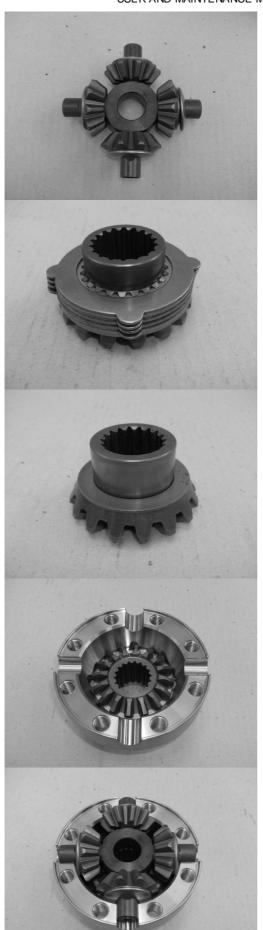
Pre-assemble the planet gears (6) with their spherical washers (5) on the spider (7).
