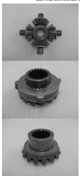
Remove the planet gears (6) and relative spherical washers (5) separating them from the spider (7).
