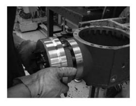
Mount the flange with drum (12) on the pinion (2).
