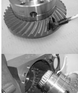
Spread a marking product, such as ink, over the bevel crown teeth to verify the goodness of the contact impression of the bevel gear teeth.
