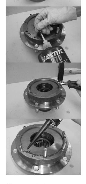
Fit the two stud bolts (4) on the wheel reduction unit and tighten at a torque of 2 daNm, applying some Loctite 270.
