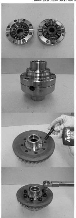
Couple the half housing (11) to the half housing (10), observing the matching as indicated in the figure.
