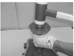
Drive the ball bearing (6) into place in the cover of the 1 speed gearbox (5) with the driver
