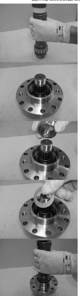
Drive the tapered roller bearing (4) on to the bevel pinion (2) with the driver.
