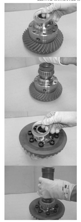
Place the necessary shims (15) on the side opposite the pre-assembled differential housing's bevel crown.
