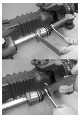
Turn the steering tie rod as illustrated in the figure to achieve bar parallelism: with one wrench hold the cylinder piston rod perfectly still while with the other wrench tighten/loosen the internal thread of the steering tie rod.
