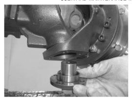
Fit the bottom knuckle pin (12) with its gasket (13) after having spread grease over it, tightening the screws (10) at a torque of 5.5 daNm and applying some Loctite 270.
