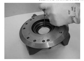
Remove the sealing ring (7) from the knuckle (8) with a screwdriver.
