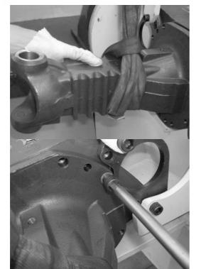
Put the axle on supports able to withstand the weight of the central body and the two lateral beams even after they have been separated or anchor the three units individually with ropes or belts to a lifting system.
