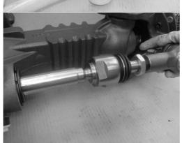
Unscrew the steering tie rod (4) from the steering cylinder piston rod (1).
