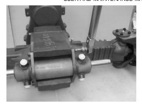
Remove the securing screws (2) of the steering cylinder (1) to the central housing and recover it.
