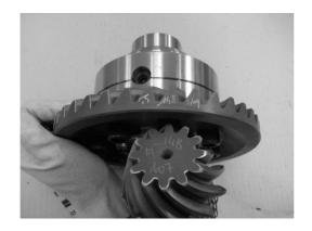
Read value "X" printed on the head of the bevel pinion (2).
