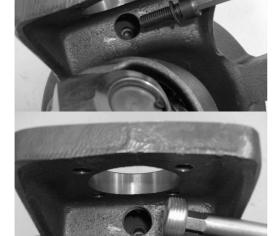
Fit the securing screw (2) with washer (2\*) under the knuckle pin housing (12) at a torque of 5.5 daNm and with some Loctite 270.
