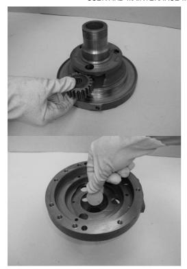
Remove the planet gear (11), putting the two axial washers and needles to one side.
