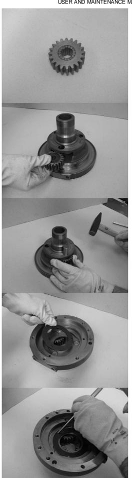
Pre-mount the needles adhering to the planet gear with grease (11).
