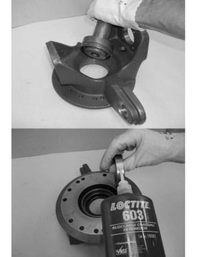
Fit the sealing ring (7) with the special tool (T02) on the knuckle (8) after having spread the lip seal with some Polymer 400 grease.
