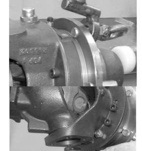
ATTENTION fasten the steering wheel reduction assembly to a suitable support.
