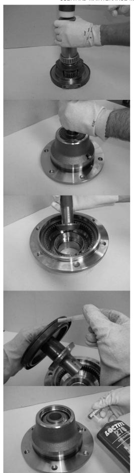
Drive the tapered roller bearing (13) into the spindle tang (8) with a driver.
