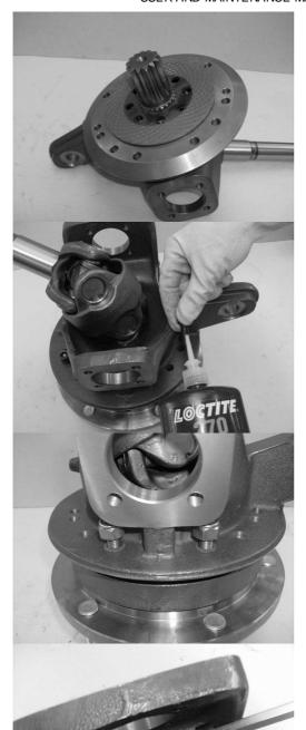
Mount the brake disc (14) on the grooved profile of the double joint.
