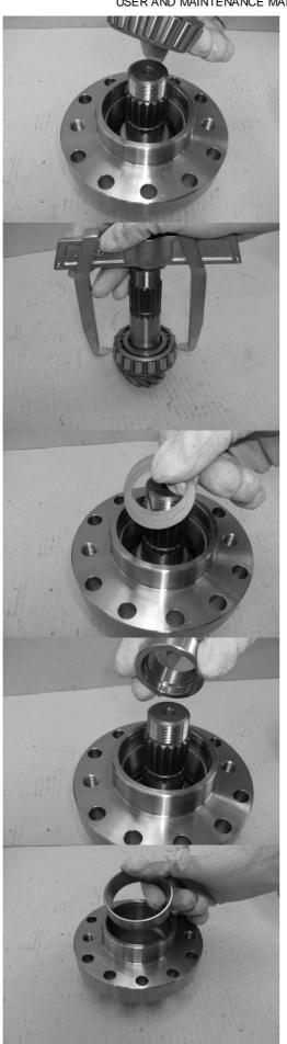
Recover the tapered roller bearing (10).
