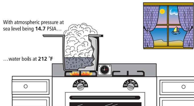
Figure 9: Saturated (Boiling) Water at Sea Level
