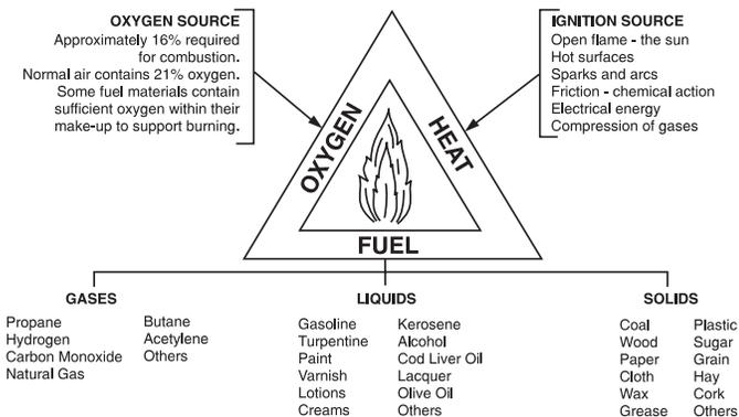
**Figure 1:** Fire/Combustion Triangle
