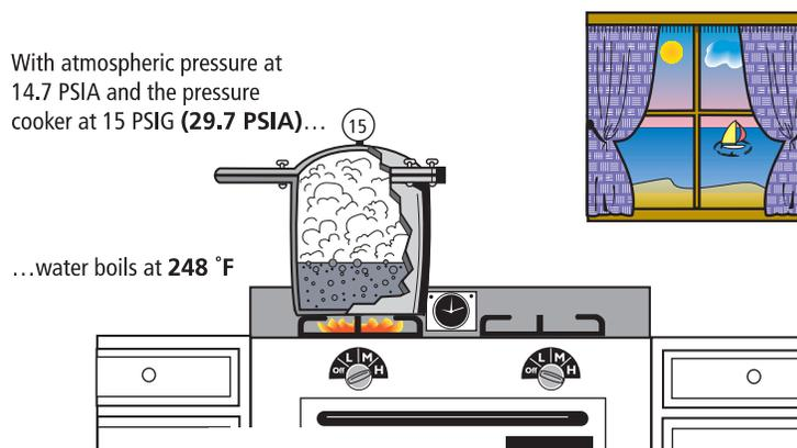
Figure 10: Saturated (Boiling) Water at Higher Pressure
