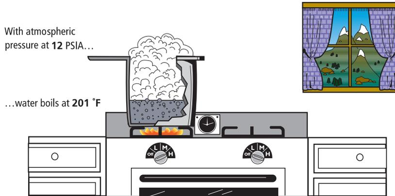
**Figure 11:** Saturated (Boiling) Water at Lower Pressure
