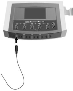
11. Plug the electrode cable(s) into the channel(s) corresponding to the channel(s) that you have programmed.
