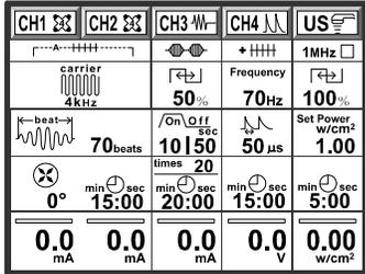
2. When you first turn the Sonicator Plus 940 on, the default parameters for each of the four stimulation channels and the ultrasound channel are displayed.
