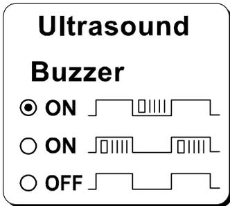
15. The “Ultrasound Buzzer” controls when the double beeps occur during a treatment as follows:
