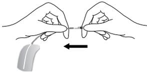
16. Plug each cable into two electrodes.
