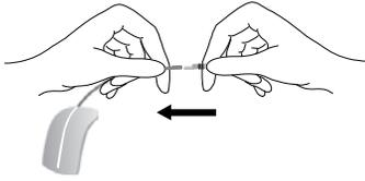
10. Plug the cable into two electrodes.
