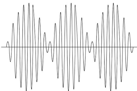
Figure 9.8—2-Pole Interferential Waveform
