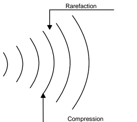
Areas of compression and rarefaction of the molecules form high frequency sound waves. Ultrasound exhibits certain beaming properties and can be reflected, refracted, scattered or absorbed. In passing through media, it is attenuated and the absorbed energy is transformed into heat. The attenuation coefficient for longitudinal waves in liquid and soft tissues is high, producing the phenomenon at bone surfaces known as selective heating.
