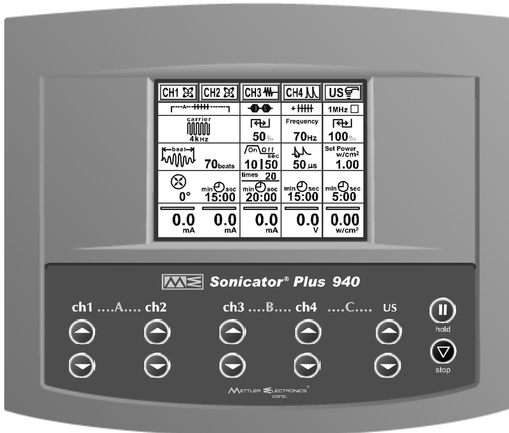
Figure 4.1 – Membrane panel and touch-sensitive screen
