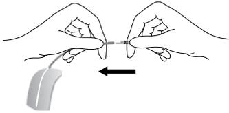
12. Plug each cable into two electrodes.
