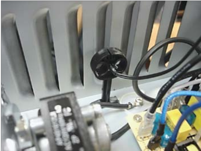
Figure 23, temperature sensor location
