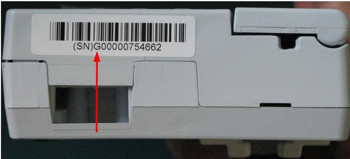
The 802.1b/g Wireless Battery Module (P/N 35162) is only compatible with pumps that include a 'G' preceding the serial number, as shown above. The 802.11b/g Wireless Battery Module (P/N 35162) should NOT be used with pumps that do not include a 'G' preceding the serial number.
