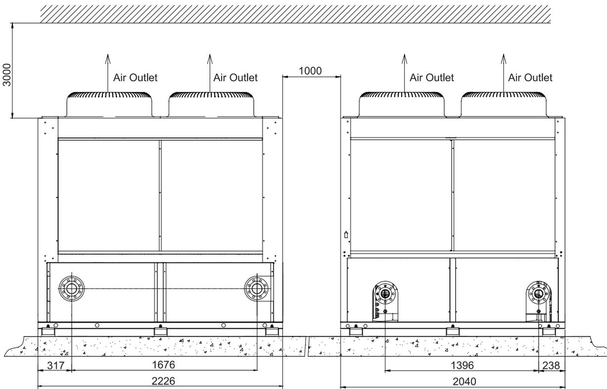
Rubber cushion pad shall be attached under the unit base which shall be fixed on the foundation with bolts.
