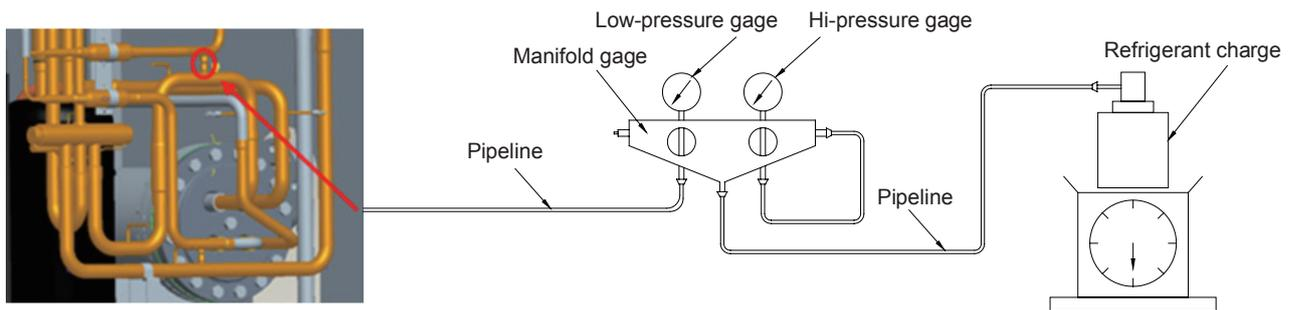
Refrigerant charge is determined through stringent tests, as excess or shortage of refrigerant would cause the compressor to run improperly. Thus, the refrigerant charge shall be consistent with that specified on the nameplate. If refrigerant charge is indeed insufficient, follow the steps below for adding.
