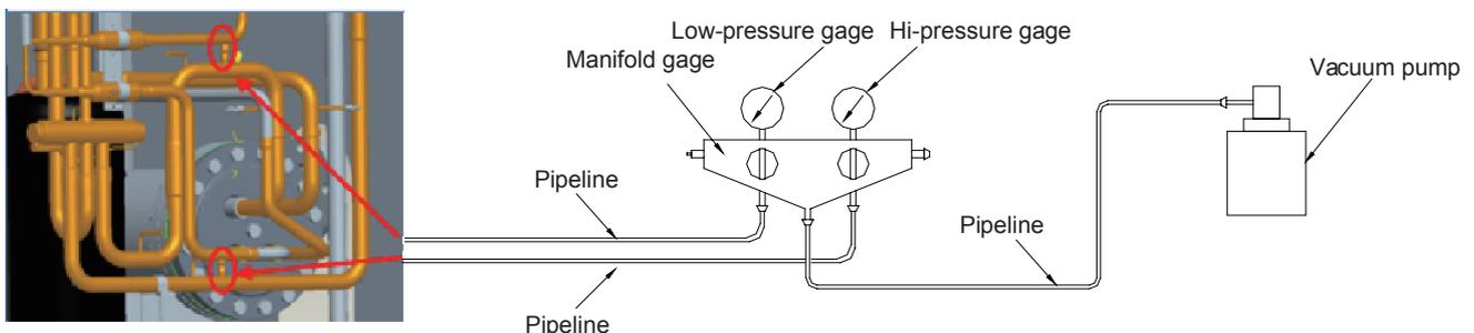
Step 3: Open the valves at both the high-pressure and low-pressure sides and then start the vacuum pump until the gage reading is below -1bar. After that, let the vacuum pump lasts for another 0.5~1.0 hour.
