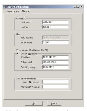
• When the Remote Enabling is ready, please verify, on the processors control panel, (by scrolling to the IP address marked with [ ) that the IP address now listed is identical to the one added in 'Static IP address' in the Remote Enabling System.
