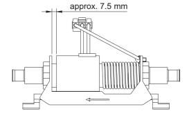
Loosen the nut (1) and adjust the screw (2) on the bottom of the pump bracket to set up the correct amount of gum by moving the coil of the pump forward or backward.
