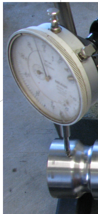
Figure 8 Dial Indicator Position for Crankshaft & Prop Flange Run Out
