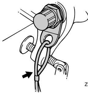
3. Secure the clamp bracket to the transom using the bolts provided with the outboard (if packed). For details, consult your Yamaha dealer. **WARNING! Avoid using bolts, nuts or washers other than those contained in the engine**
