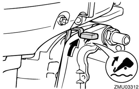
3. Slightly tilt the outboard motor up. The tilt support bar will lock automatically, supporting the outboard motor in a partially raised position. This outboard motor has 2 positions for shallow water cruising.
