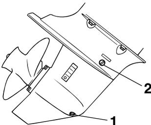
1. Gear oil drain screw
