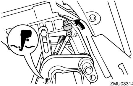
2. Slightly tilt the engine up until the tilt support bar is automatically released.
