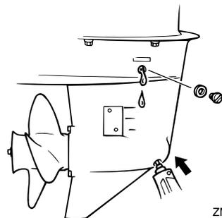
6. Put a new gasket on the oil level plug. When the oil begins to flow out of the oil level plug hole, insert and tighten the oil level plug.
