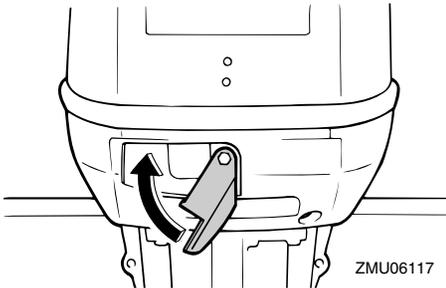
After installing, check the fitting of the top cowling by pushing it with both hands. If the top cowling is loose, have it repaired by your Yamaha dealer.
