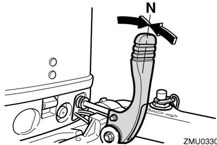
2. Place the tilt lock lever in the release/up position.
