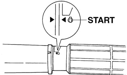
4. Pull out / turn the choke knob fully. Place the choke knob back in to the second or third position to warm up the engine after starting. When the engine has fully warmed up, replace the choke knob back in to its home position.
