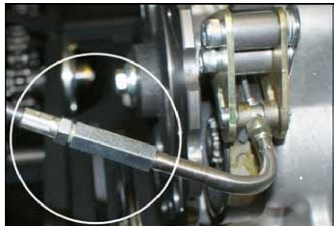
Figure 7-19c. Adjusting the parking brake.
