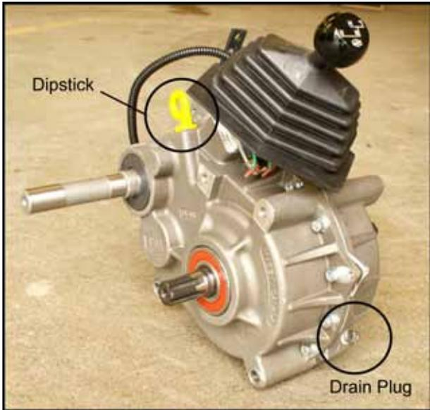
Figure 6-4a. 34-100 Transmission showing dipstick and drain plug locations
