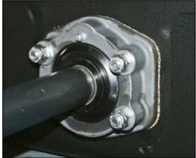
Figure 7-15. Bearing Flange and Cork Gasket
