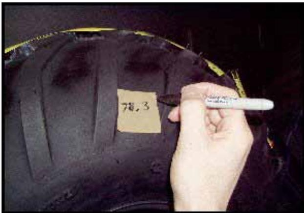
Figure 11-6. Marking the tire.
