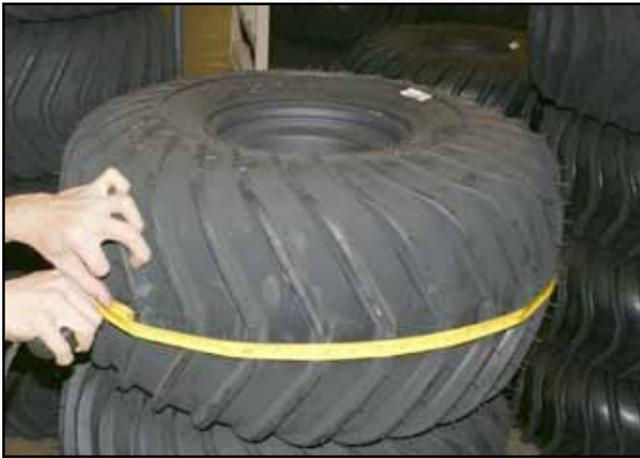
Figure 11-5. Measuring the tire.
