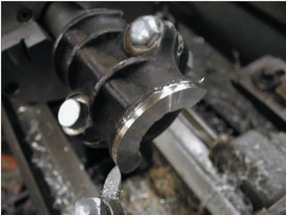
Photo 4: Squaring up the thrust surface
