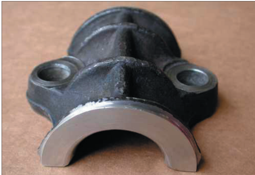
Photo 5: Finished bearing cap
