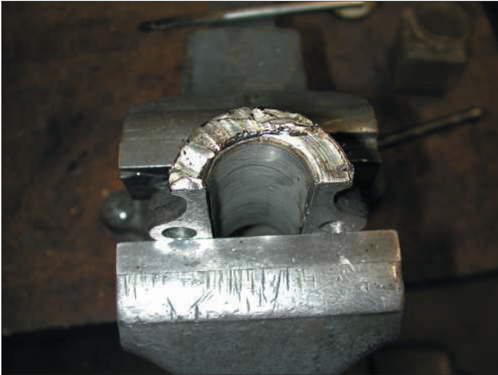
Photo 2: Adding babbitt to the thrust surface of the rear main bearing cap
