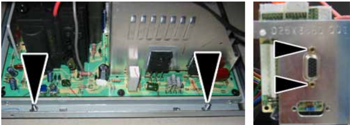
Figure 17. Removing the Monitor PCB Mounting Hardware
